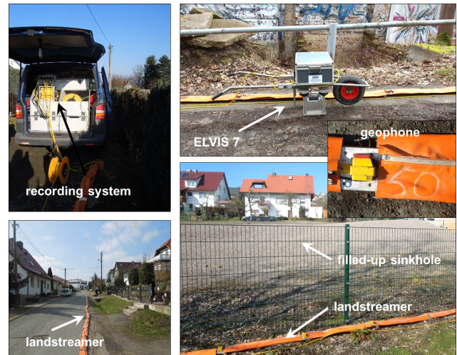
Figure 5. Photographs taken during the two field campaigns showing the micro-vibrator, the land streamer and the recording system used for the S_H -wave reflection-seismic surveys.
