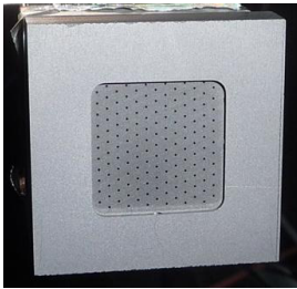
Fig. 10: Front view of the retarding potential analyser
