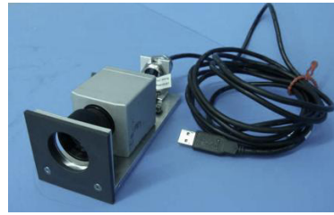
Fig. 11: Thermocamera setup with housing (without cover and window)
