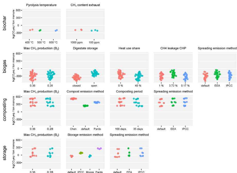
Fig. 5. Sensitivity of net greenhouse gas emissions to parameters assumptions. Depicted are only the variants with 10 km transport from processing to field. The unit of the maximum CH 4 production potential ( B_0 ) varied for biogas, composting and storage is m^3 CH 4 /kg manure oDM.
