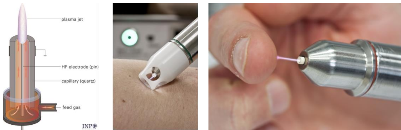
Figure 6. The approved (medical device class IIa) atmospheric pressure argon plasma jet kINPen MED. Current medical indications are decontamination and promotion of wound healing. (Left) Scheme of a prototype of the kINPen plasma jet with argon gas used as feed gas that is excited in a high-frequency electrode before driven out into the ambient air to generate reactive oxygen and nitrogen species. (Middle) kINPen MED equipped with a space. (Right) kINPen MED plasma jet connecting to the skin. Image reproduced from [93].
