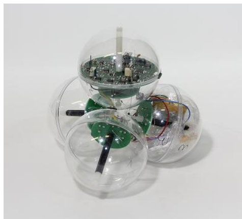
Figure 3. The completely assembled air speed measuring device.
