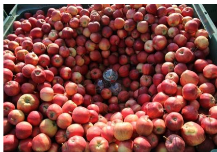
Figure 13. Position of the device for airspeed measurement between apples in a storage bin.
