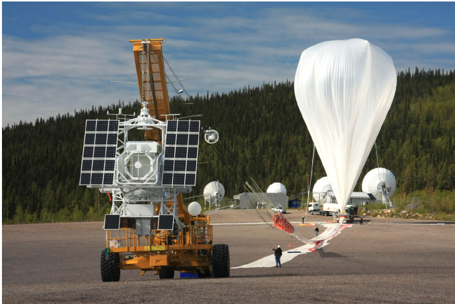
Figure 14 Sunrise immediately before launch. The balloon is only partly filled on ground to allow expansion with decreasing outside air pressure during ascent. At 37 km altitude it will have expanded by a factor of 300 as compared to ground. The parachute for landing is part of the flight train connecting the gondola payload with the balloon.
