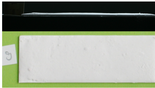
Figure 4. Glass substrate with a \text{CaCO}_3 layer (side and front view).
