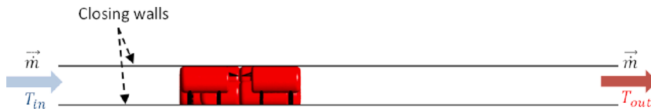
Fig. 4. Configuration for heat transfer evaluation in close domain.
