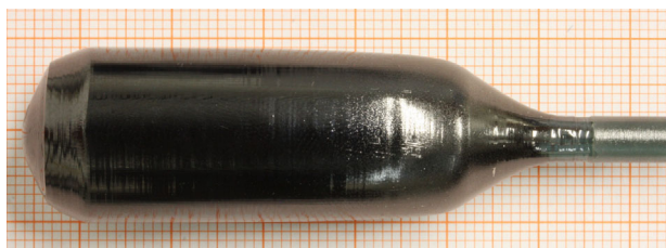
Figure 1. Typical NdScO 3 crystal grown at IKZ with a cylinder length and diameter of around 40 and 18 mm, respectively.
