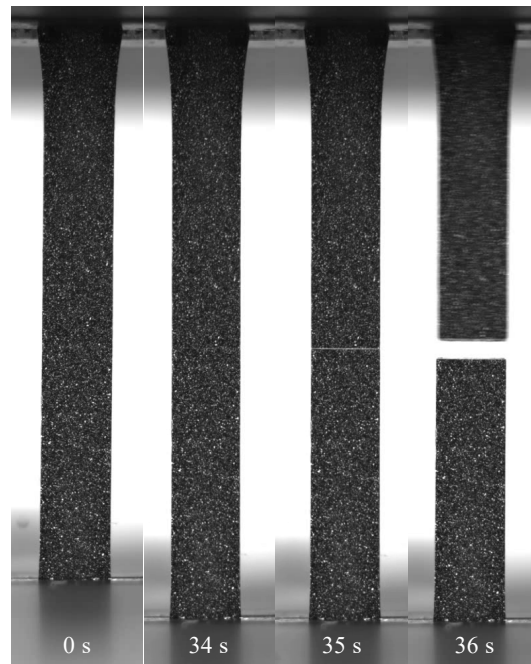
Figure 19. Deformation progression of a WL specimen of 1.8-CB/30-CC/0.25-SP under DIC.
