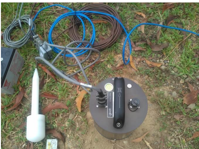
Figure 3. Guralp 6TD/Broadband seismometer, break out cable, GPS antenna, and battery for power supply
