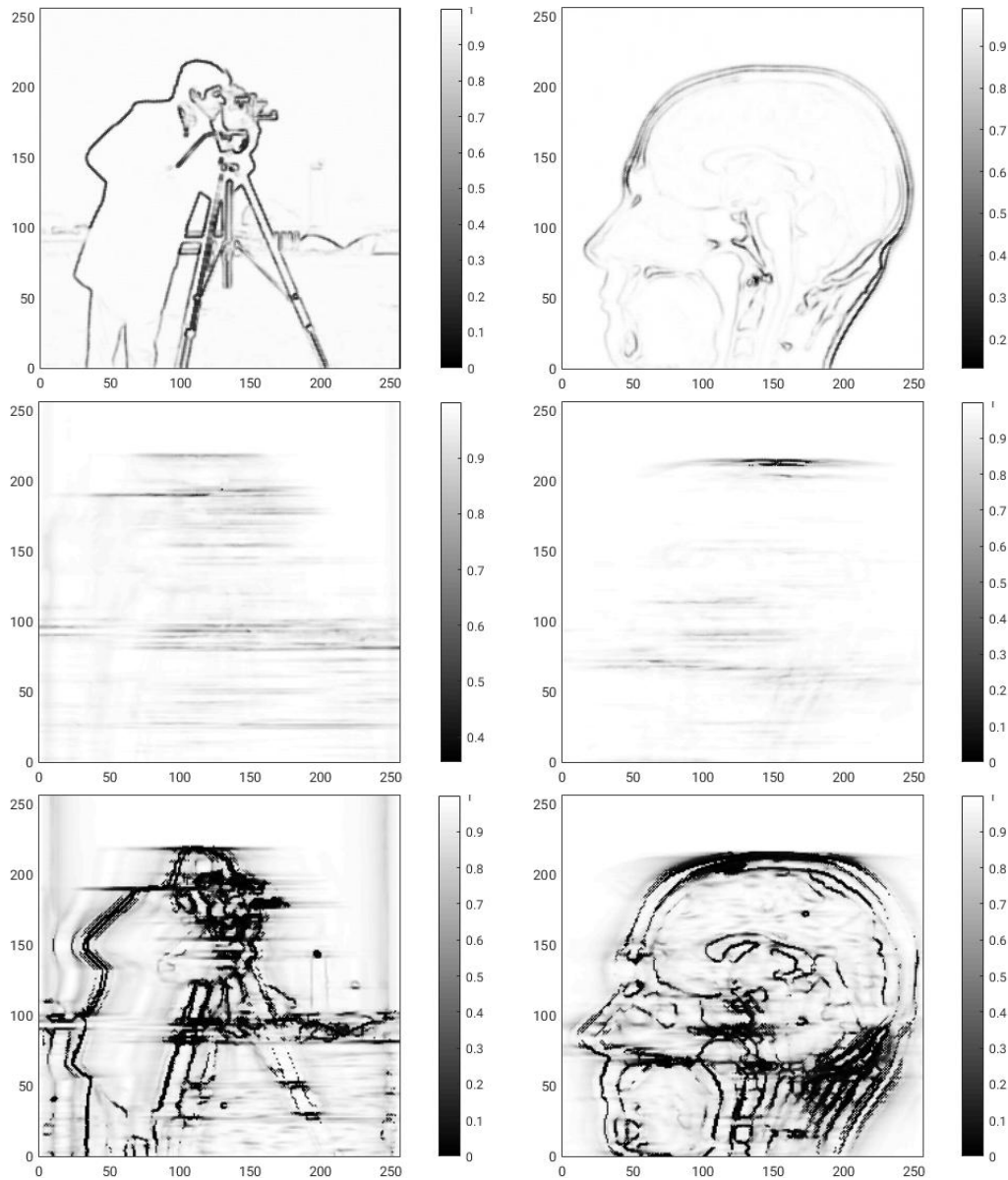
Figure 4: Numerical results for the quantiles. Top row: white noise model with s = 0.9 , Middle row: motion blur model with s = 0.5 , Bottom: motion blur model with s = 0.1 Left: Cameraman, Right: MRI.
