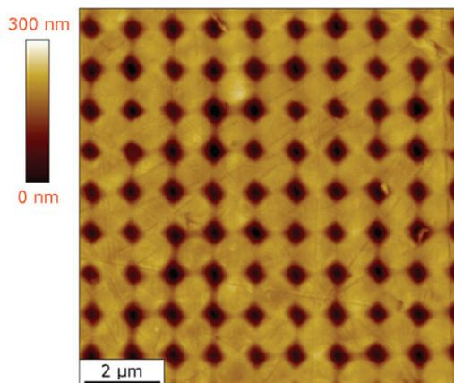
Fig. 7. AFM image of the copper surface after laser embossing with master foil (A)
