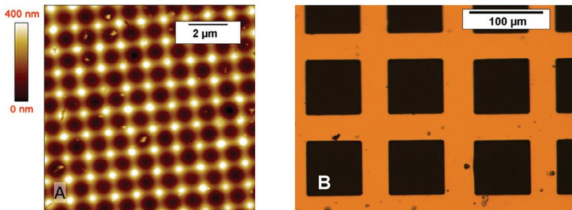
Fig. 1. (Left) AFM images of the nickel foil used as master form (A), (right) optical microscope image of the nickel foil used as master form (B)
