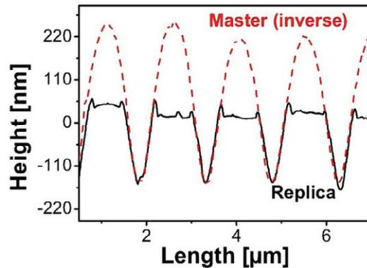
Fig. 8. Depth profile of the inverse master form (nickel foil (A), Fig. 1) and the replicated structures in the copper workpiece (Fig. 7) – measured with AFM
