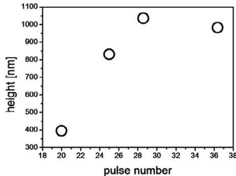
Fig. 5. Heights of the replicated structures in the copper workpiece in dependence on the applied laser pulse number. Nickel foil (B) was used as master form. The laser fluence used was  $F = 3.7$  J/cm<sup>2</sup>
