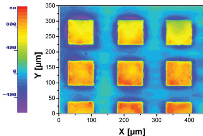
Fig. 3. Image of the copper surface taken by WLI after the laser embossing with nickel foil (B)
