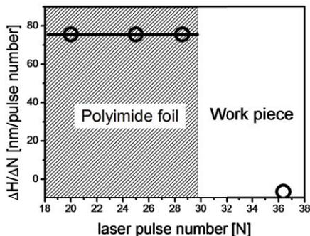
Fig. 6. Differential height changes of the formed structures in the copper workpiece in dependence on the applied laser pulse number. The shaded area indicates that the applied laser pulses are absorbed in the polyimide foil. In the blank area the laser pulse irradiated the nickel foil and parts of the copper workpiece
