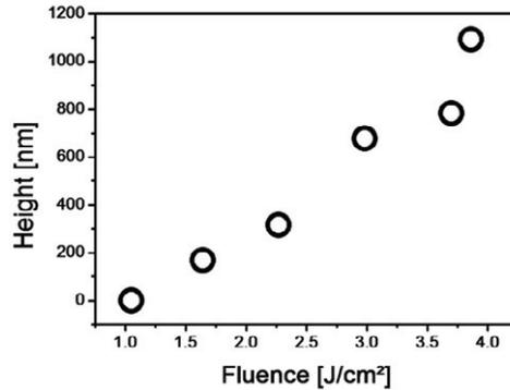
Fig. 4. Heights of the replicated structures in the copper workpiece in dependence on the used laser fluence. Nickel foil (B) was used as master form. The laser scanning speed was  $v = 1.4$  mm/s which is equal to 29 laser pulses per point
