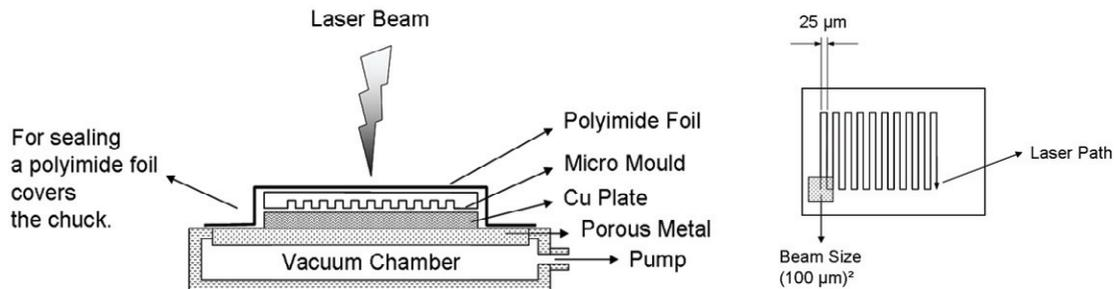
Fig. 2. (a) sketch of the experimental set-up used; (b) Scanning path of the laser beam across the workpiece during the laser embossing process
