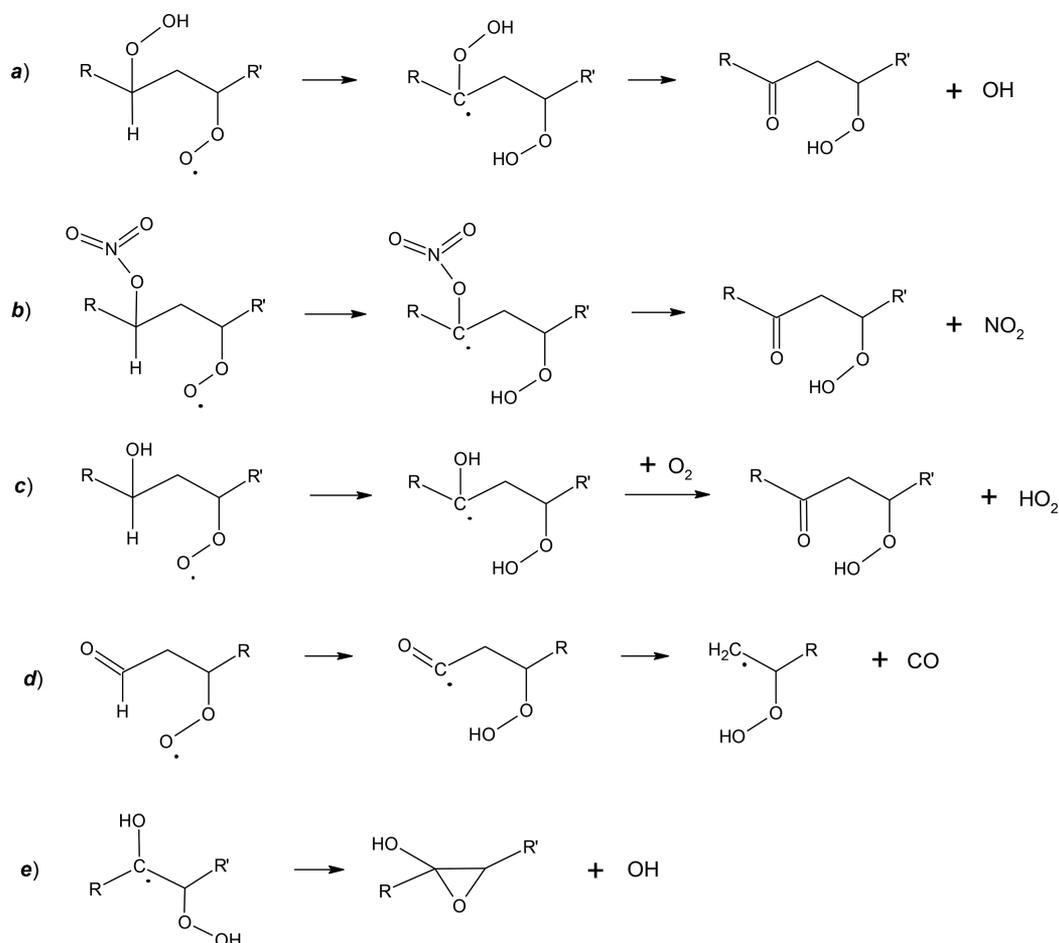
**Figure 9.** Unimolecular fragmentation reactions of peroxy radicals. (a) OH loss following H-abstraction from a carbon with a  $-\text{OOH}$  group attached. (b)  $\text{NO}_2$  loss following H-abstraction from a carbon atom with a  $\text{ONO}_2$  group attached. (c)  $\text{HO}_2$  loss following H-abstraction from a carbon atom with an OH group attached (and subsequent  $\text{O}_2$  reaction). (d) CO loss following H-abstraction from an aldehydic carbon atom. (e) Epoxide formation.
