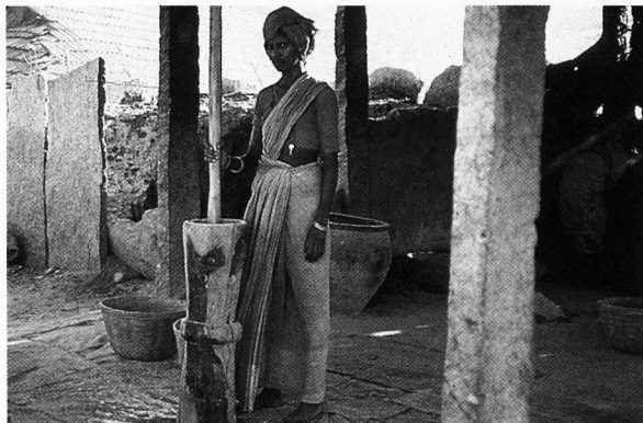
Figure 13. Together with rice dust the tumbled beads are pounded to shape with a wooden pestle in a wooden mortar, Papanaidupet.
