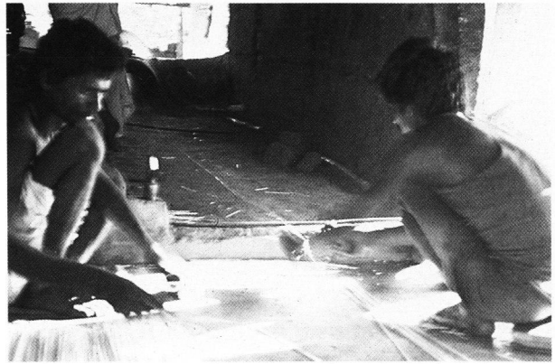
Figure 10. Drawing the glass tube. One man pulls continuously, while the other cuts off lengths of about 1.00 to 1.20 m, Papanaidupet.
