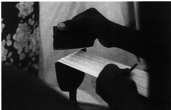
Figure 11. Cutting glass tubes of opaque white glass to bead-size slices. The slices are caught in a sheet.
