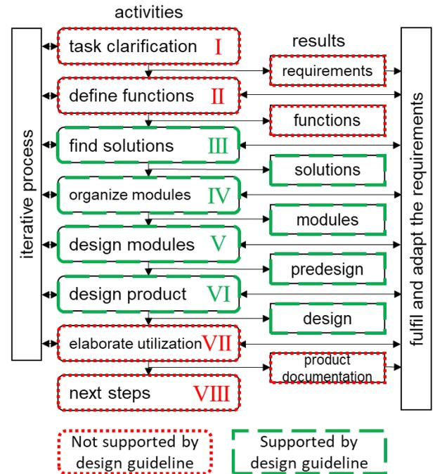
Figure 5. Integration of the design catalogues into the VDI 2221 [15]
