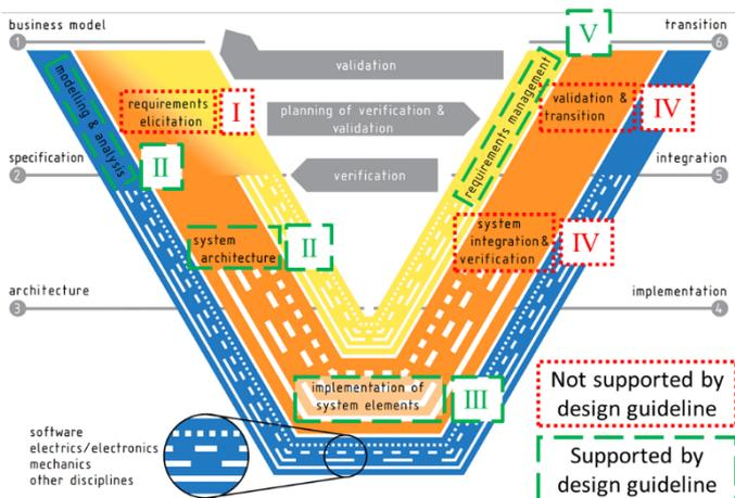
Figure 4. Integration of the design catalogues into the V-model of VDI 2206 [14]
