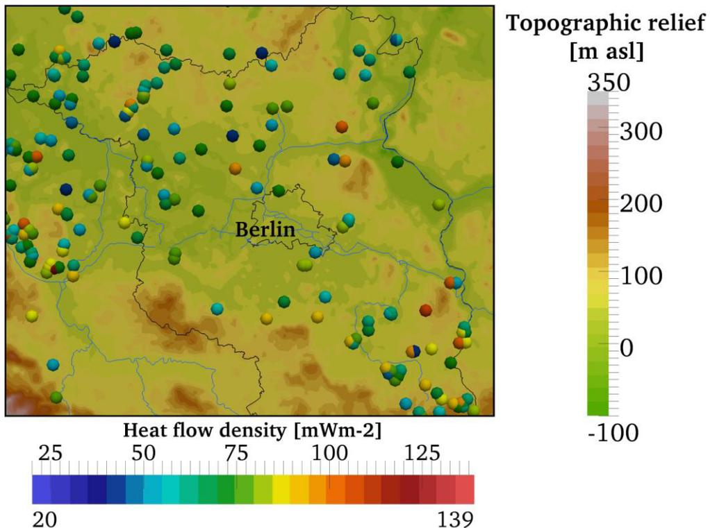
Fig. 1. Heat Flow density measurements as extracted from the heat flow database for Germany as provided by the Atlas of Geothermal Resources in Europe, Hurter and Haenel [1]. The background map shows the topographic relief in the area
