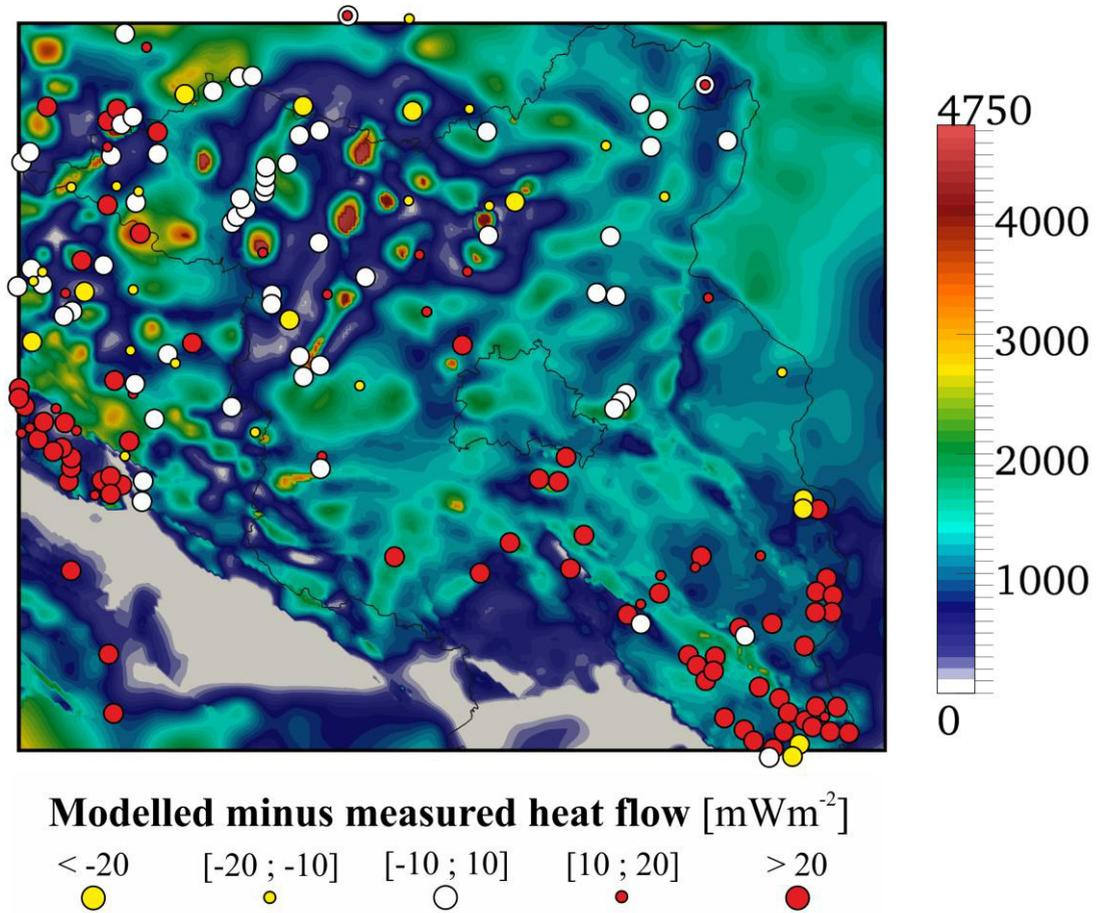
Fig. 3. Differences between modelled and measured heat flow values. The background colour map indicates the thickness of the Zechstein salt layer
