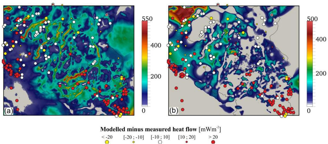
Fig. 4. (a) Differences between modelled and measured heat flow values. The background colour map indicates the thickness of the Quaternary layer. (b) Differences between modelled and measured heat flow values. The background colour map indicates the thickness of the Rupelian Clay
