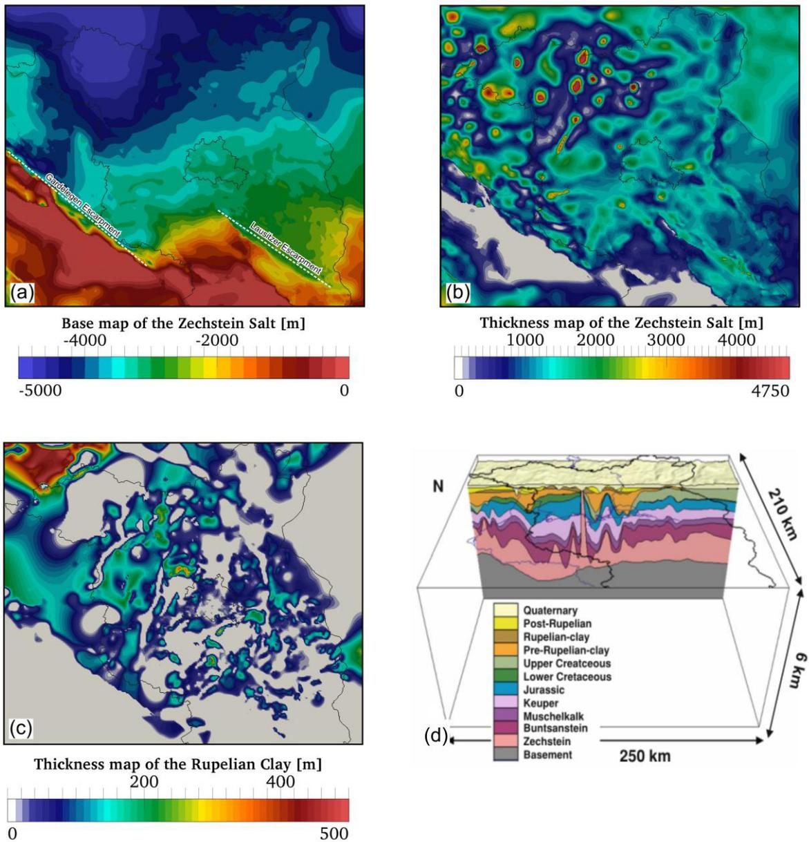
Fig. 2. (a) Depth to the base of the Zechstein salt. Also shown by dotted white lines are the approximated traces of the two major fault zone along the southern margin of the basin. (b) Thickness map of the Zechstein salt. (c) Thickness of the Rupelian Clay. (d) 3D view of the geological model for the sedimentary layers as used for the heat flow calculation, after Noack et al. [2]. Different colours indicate the distinct stratigraphic units
