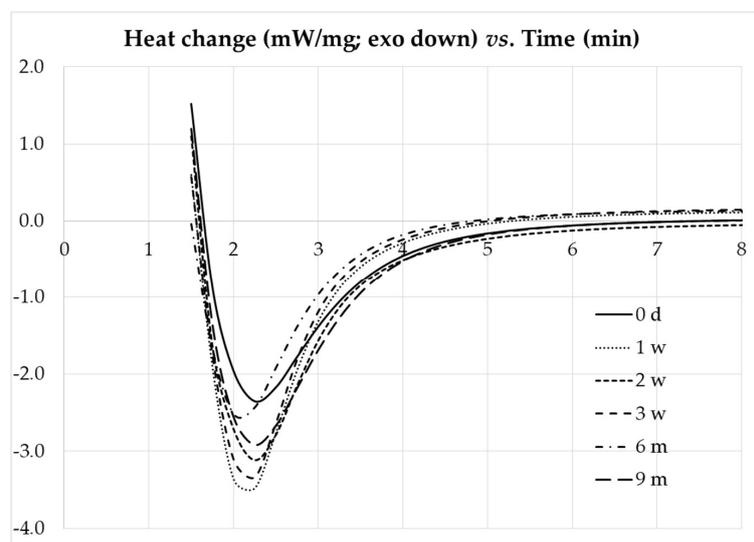
**Figure 14.** DSC isothermal profiles of composite with different storage times.
