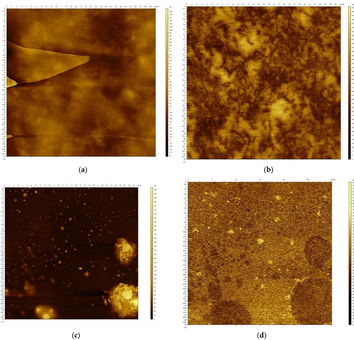
**Figure 7.** AFM images of the epoxy composites with 1.2 wt.% SWCNT (a,b) and 5 wt.% EG (c,d). Images (a,c) were obtained in topographic mode while b and d were obtained in high definition kelvin Force microscopy (HD-KFM) mode.
