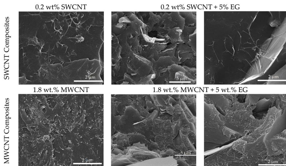
**Figure 5.** SEM micrographs of selected epoxy nanocomposites.
