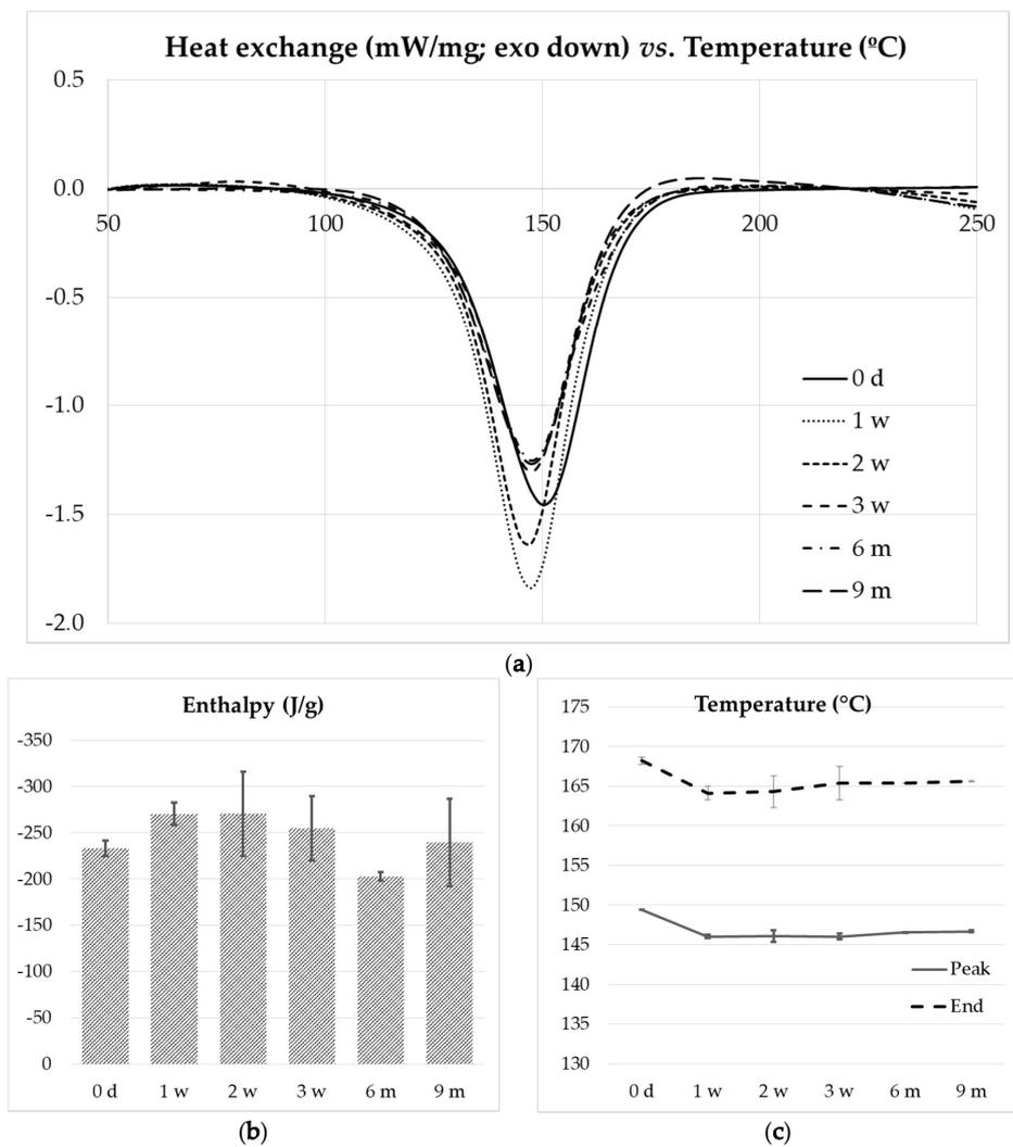
**Figure 13.** DSC profiles for scans at 10 °C/min of composites with 0.5 wt.% SWCNT + 2 wt.% EG after different storage times. (a); corresponding cure enthalpies and (b); peak temperatures and peak end temperatures (c).
