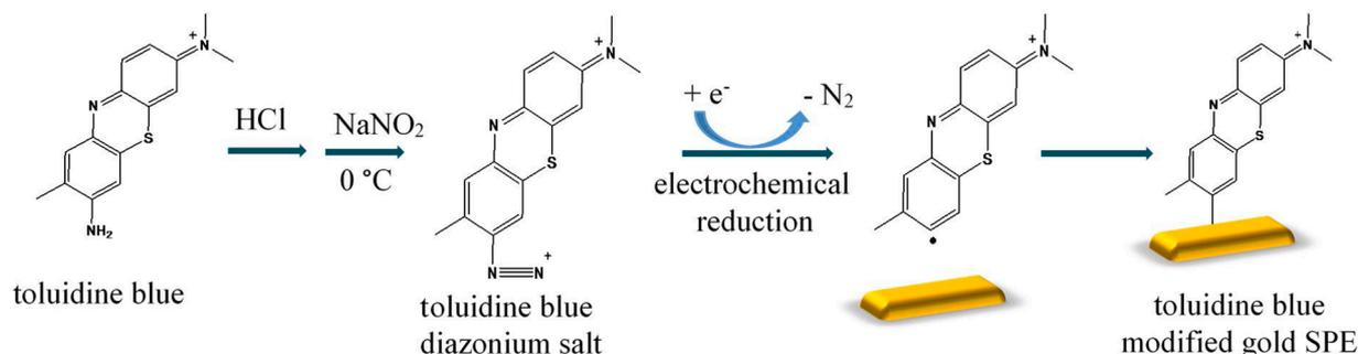
Scheme 1. Synthesis and electrografting of TB diazonium salt onto the gold SPE.
