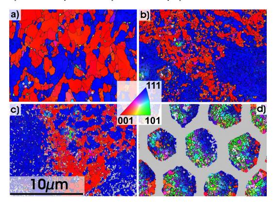
**Figure 5.** Fraction of different fibre texture components. Overlaps between components are possible since values summed up within  $\pm 20^{\circ}$  around the particular ideal orientation.
