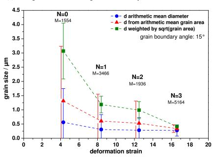
(b) mean grain diameter for grains estimated by three different method.
