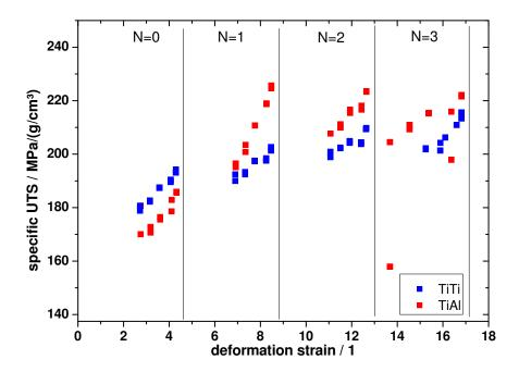
It can be seen that the Ti-Al wires are superior to Ti-Ti wires that have identically been deformed.
