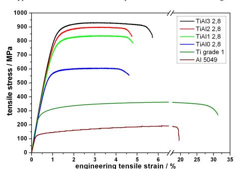
**Figure 8.** Typical stress-strain curves for the produced wires and the starting materials.
