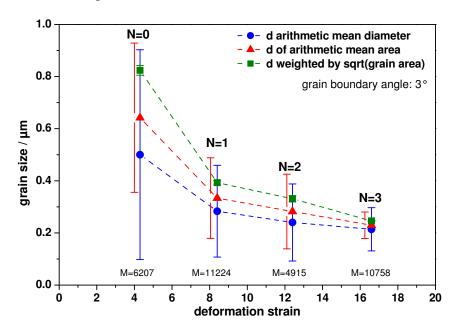
(a) mean grain diameter for subgrains estimated by three different methods.
