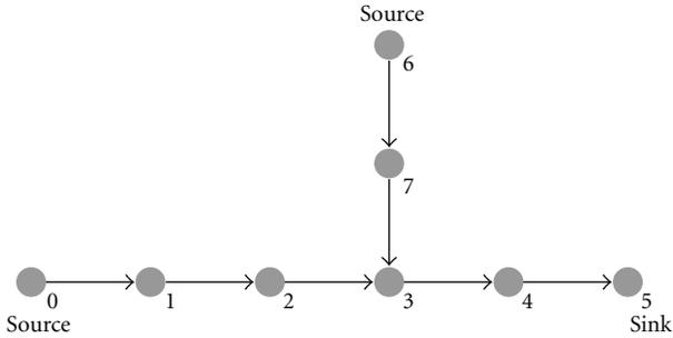
FIGURE 21: Two sources—nodes 0 and 6—send data periodically to the sink (node 5).
