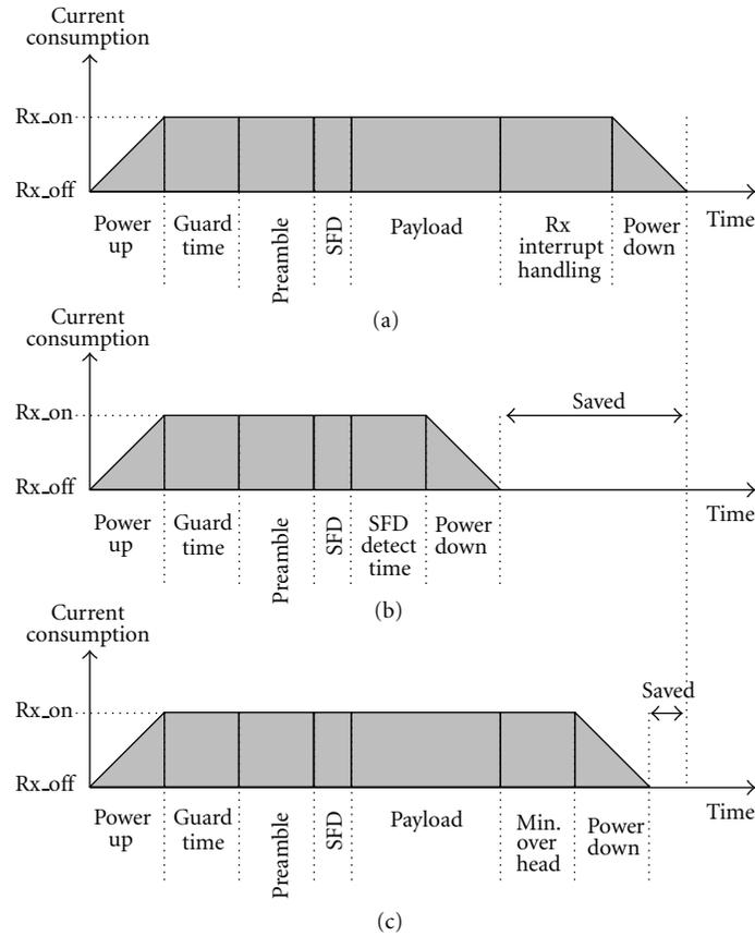
FIGURE 17: (a) General receive slot (software only). (b) Shortened passive slot with ILA and ASIC. (c) Active slots with reduced idle listening (ASIC only).
