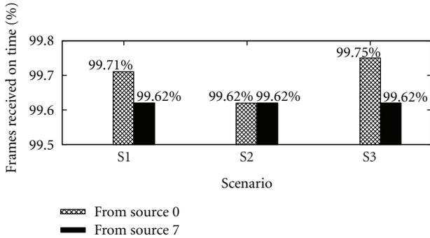
FIGURE 25: Small network: the number of frames (event notices) the sink received on time; it does not include missed frames.
