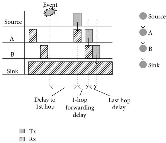
FIGURE 3: Nodes with staggered (aligned) schedule forwards frames just after reception and reduce end-to-end delays.
