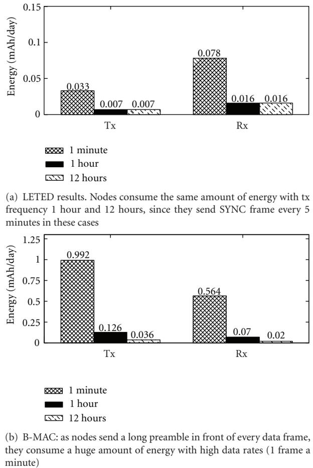
FIGURE 33: Energy of data transmission and reception for various data rates (a frame sent every 1 minute, 1 hour, and 12 hours) when supporting 5-second end-to-end delays.
