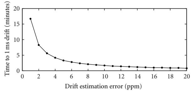
FIGURE 11: LETED slots move by 1 ms due to errors in drift estimation after the time depicted here.
