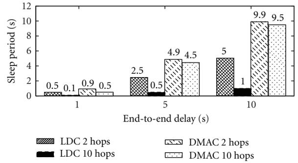
FIGURE 4: To support short end-to-end delays, nodes with common low duty cycle (LDC) protocols wake up often, especially when the distance between sources and the sink is long; DMAC introduces the staggered schedule and lowers the duty cycle; that is, nodes wake up more rarely than in common LDC protocols to support short delays; besides, with DMAC the distance to the sink only slightly impacts the duty cycle.
