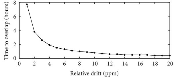
FIGURE 14: Average time to slot overlap, beacons or LETED slots, of nodes having four neighbors and a schedule supporting 10-second delays for different clock drift values.
