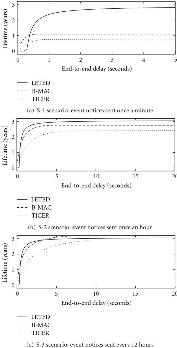
FIGURE 32: The lifetime of nodes with LETED and with Preamble Sampling (B-MAC and TICER).
