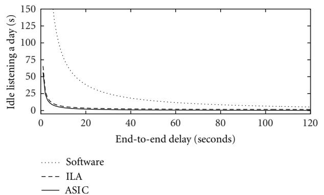
FIGURE 19: Idle listening causes by LETED of three various solutions: software, based on Tmote Sky (ILA) and with a dedicated hardware (ASIC).
