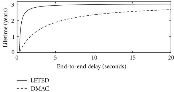
FIGURE 38: Lifetime of LETED and DMAC; owing to idle listening avoidance (ILA), LETED shortens significantly passive slots, saves the energy, and prolongs the lifetime.
