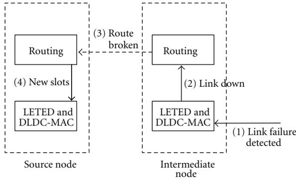
FIGURE 16: When a node detects a link failure (at the MAC level), it triggers the network layer (routing) to find a new path; a *route broken* message is sent to the source, which discovers another route and establishes a schedule along the new path.
