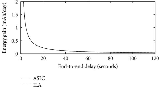
FIGURE 20: Energy gain of solutions to idle listening avoidance based on hardware: ILA (with CC2420 transceiver) and ASIC (based on dedicated hardware); as both solutions achieve similar results, the difference between them can hardly be spotted in this figure.
