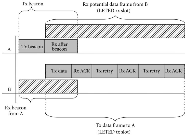
(a) Slot overlap risk: Tx beacon of node A overlaps with LETED slot from B to A
