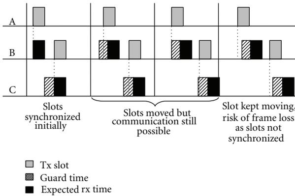
FIGURE 10: Nodes shift slots according to relative drift to the source. Because of errors in multihop drift estimation, they shift slots by different times. Thus, slots of senders and receivers drift away.
