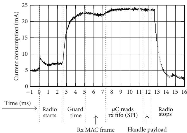
FIGURE 18: Rx slot of Tmote Sky sensor node (oscilloscope output: average from 2 samples); MAC frame 62 bytes data rate 250 kbps.
