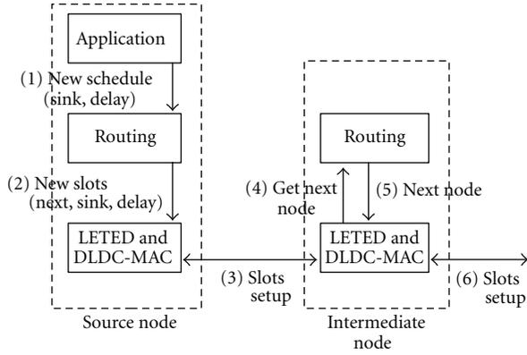
FIGURE 7: Setup of a new wake-up schedule; application triggers the network layer (routing) to set up a new schedule to the sink; on each node, the network layer (routing) requests MAC to establish time slots to the next node.
