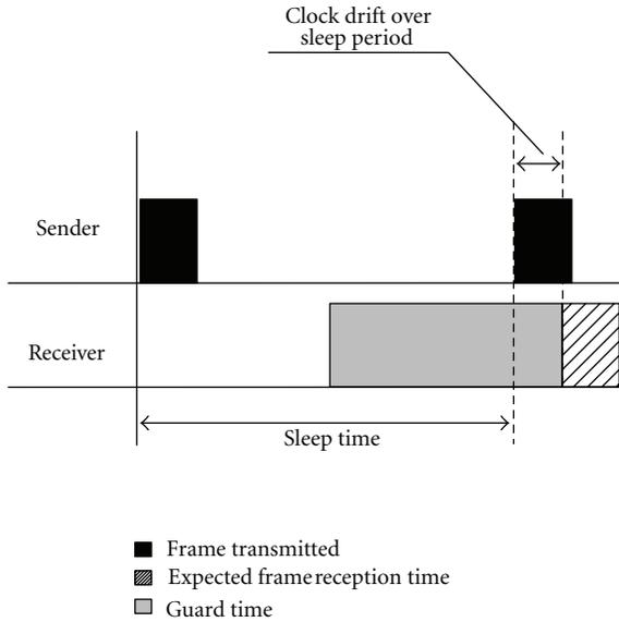
FIGURE 6: To compensate clock drift receivers wake up earlier by guard times.
