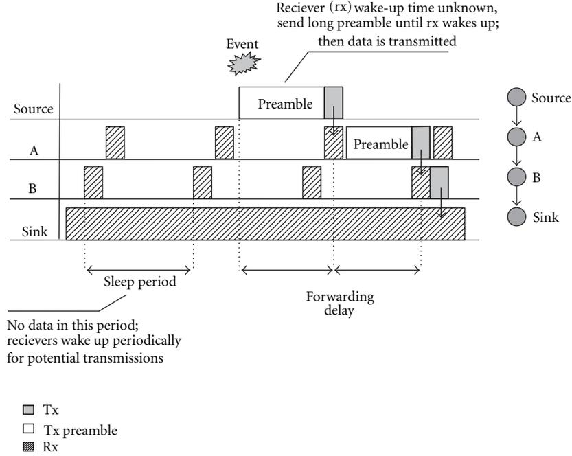
FIGURE 5: With preamble sampling (cycled receiver) nodes send long preambles in front of frames and receivers check periodically for transmissions. The length of preamble and of sleep periods impacts end-to-end delays resulting in significant end-to-end delays.
