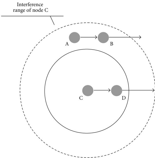
FIGURE 13: Although both paths are out of their transmission range, they are within the interference range and affect each other.
