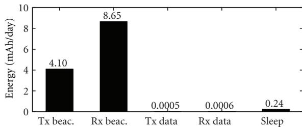
FIGURE 36: DLDC-MAC energy consumption; short sleep periods (1 second here) and a long time of beacons transmission and reception (about 12 ms altogether) result in an excessive energy waste.
