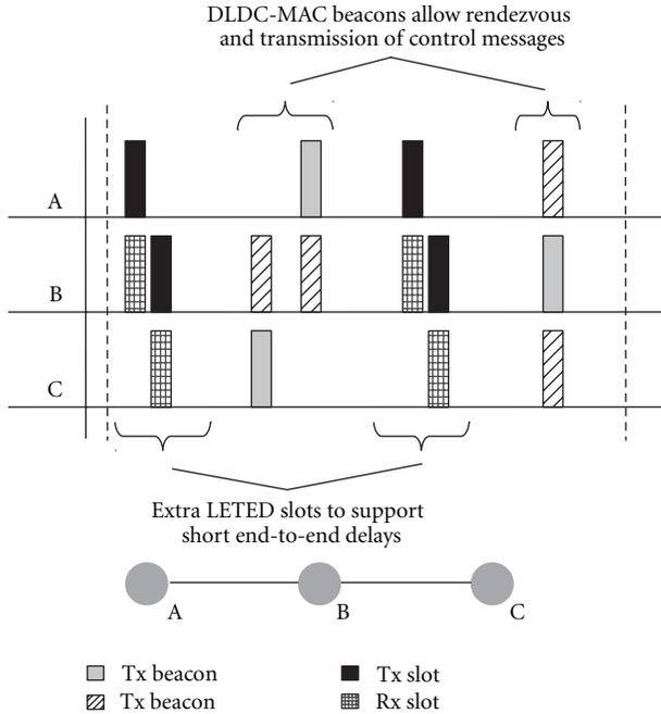
FIGURE 1: With DLDC-MAC nodes send periodically beacons and wake up to receive beacon from neighbors; to support short end-to-end delays nodes apply extra LETED slots.
