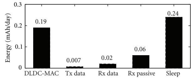
FIGURE 37: Energy consumed by LETED; owing to Idle Listening Avoidance nodes consume little energy while waiting for potential transmissions (Rx passive).
