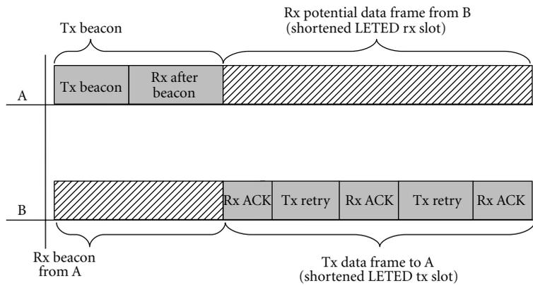
(b) Joined slots: after beacon finishes there, nodes A and B use the rest of the LETED slot
