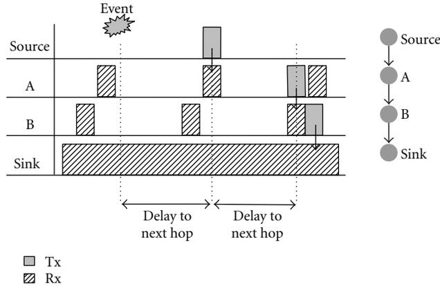
FIGURE 2: By applying low-duty cycle protocols, nodes mostly sleep and cannot forward data immediately but wait until the next node is awake. It causes significant end-to-end delays.
