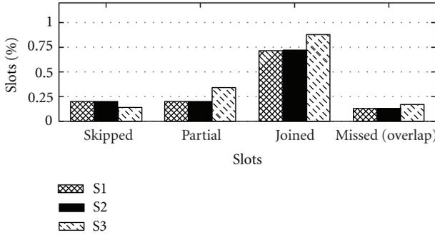
FIGURE 29: Small network: the number of slots skipped, used partially, and joined upon an slot overlap risk among all nodes, for each test run separately.
