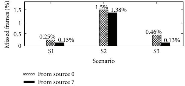
FIGURE 26: Small network: the total number of event notices that the sink did not receive, that is, end-to-end packets, for each source separately.
