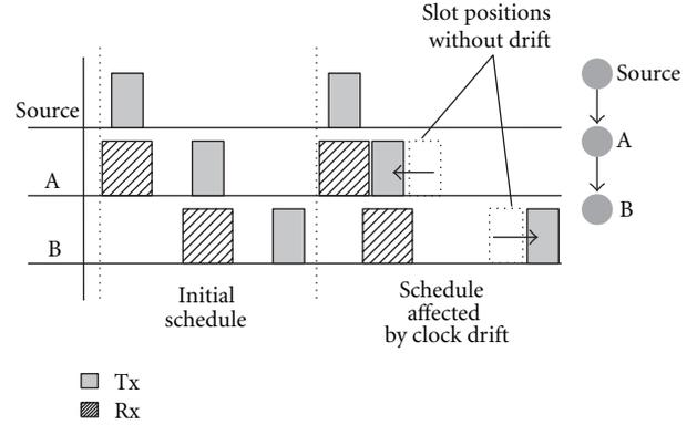
FIGURE 8: Due to clock drift, slots of different nodes move relatively to each other.
