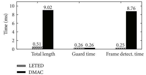
FIGURE 40: Passive slots consist of guard times that compensate clock drift and the time needed to detect that no frame arrives in the current slot.
