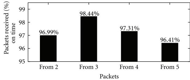
FIGURE 27: Large network: the amount of frame the sink received on time, that is, within 10 seconds.
