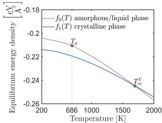
Figure 2: Minimum values for the free energy density for liquid/amorphous ( $f_0(T)$ ) and crystalline ( $f_1(T)$ ) equilibrium to the SW potential for a temperature range of 200–2000 K. The free energy equilibrium values are calculated with the codes provided by Ruy and Cai [36]. For the liquid branch,  $T_g$  points out the glass transition. The free energies for the amorphous phase were calculated by Broughton and Li [6].
