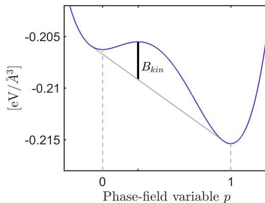
Figure 1: Example of the bulk free energy density  $F$  and its kinetic barrier  $B_{kin}$  at temperature  $400K$  (less than  $T_m$ ).  $B_{kin}$  is the kinetic barrier, that has to be overcome to pass from one phase into the other.
