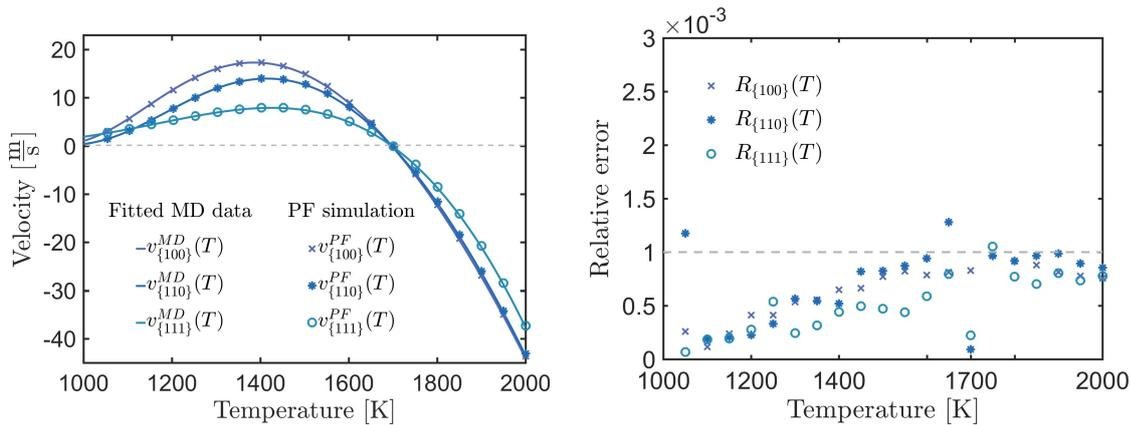
Figure 7: The points in the left figure are the measured velocities from the numerical solution of equation (11). The solid lines are the fitted velocities from molecular dynamics. Clearly, model (11) with the atomistic informed parameters reproduces exactly the kinetic interface-behavior. As shown in the right figure, only 5% of the relative errors of the velocities are greater than  $10^{-3}$ . The highest error is about 0.0013 for the  $\{110\}$  orientation at  $T = 1650\text{K}$ .
