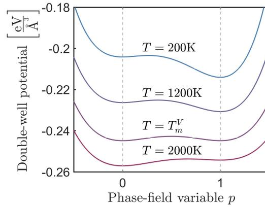
Figure 5: The double-well potential at different temperatures. At the melting point  $T_m$ , the two minima of the bulk free energy density have the same value.
