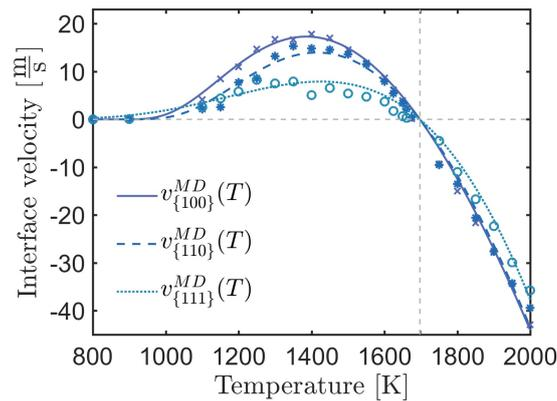
Figure 4: Crystallization velocity over temperature for silicon with the Stillinger-Weber potential, fitted by a Vogel-Fulcher equation(10).
