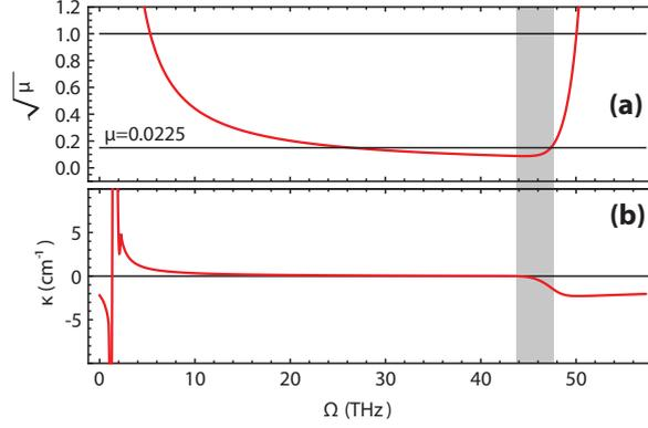
Figure 4: (a) Pairs of  $\Omega$  and relative DW amplitude  $\sqrt{\mu}$  for which solitons frequency does not change. Amplitude is plotted instead of power to facilitate readability. (b) Stability analysis. The region of stable SSFS compensation is shaded gray.
