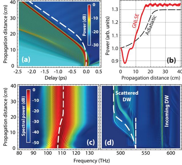
Figure 1: GNLSE calculation of a DW at 3.67 PHz interacting with a soliton at 0.67 PHz. (a) Power in space-time domain. The white dashed line is the soliton trajectory in the adiabatic approximation. (b) Soliton peak power from GNLSE (red line) and adiabatic theory (dashed line). (c,d) spectral power for soliton and DW respectively. Dashed lines are from adiabatic equations (7–9).
