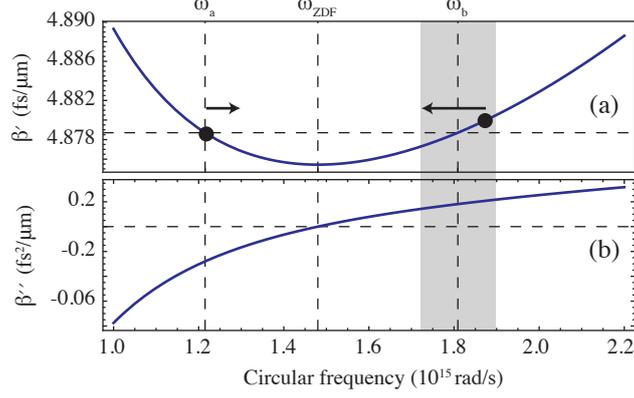
Figure 2: A typical profile (bulk silica) of (a) the group delay  $\beta'(\omega)$  and (b) GVD  $\beta''(\omega)$  that leads to the collision phenomenon shown in Fig. 1. Collision can only be realized for initial DW frequency offsets in a small interval (shaded gray) around the reference frequency of matching group velocity. Initial frequencies of soliton and DW are indicated by bullets, frequency shifts are indicated by arrows.
