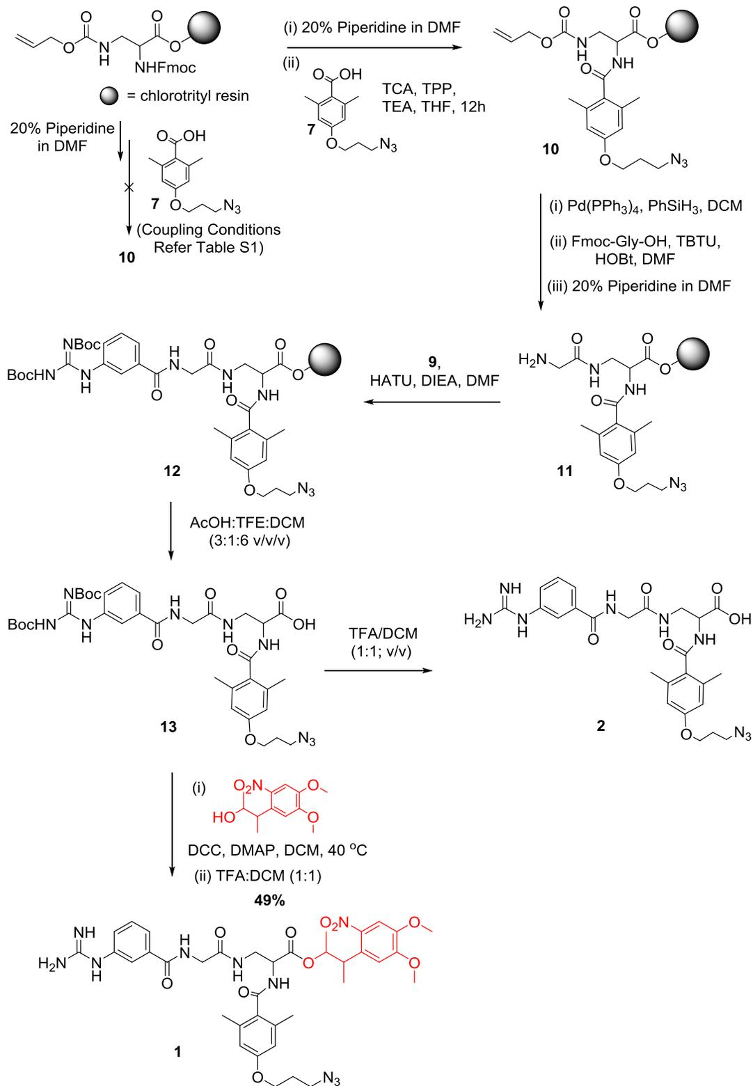
**Scheme S2:** Detailed scheme of synthesis of  $\alpha_5\beta_1$  specific ligand (2) and its phototriggerable derivative (1).
