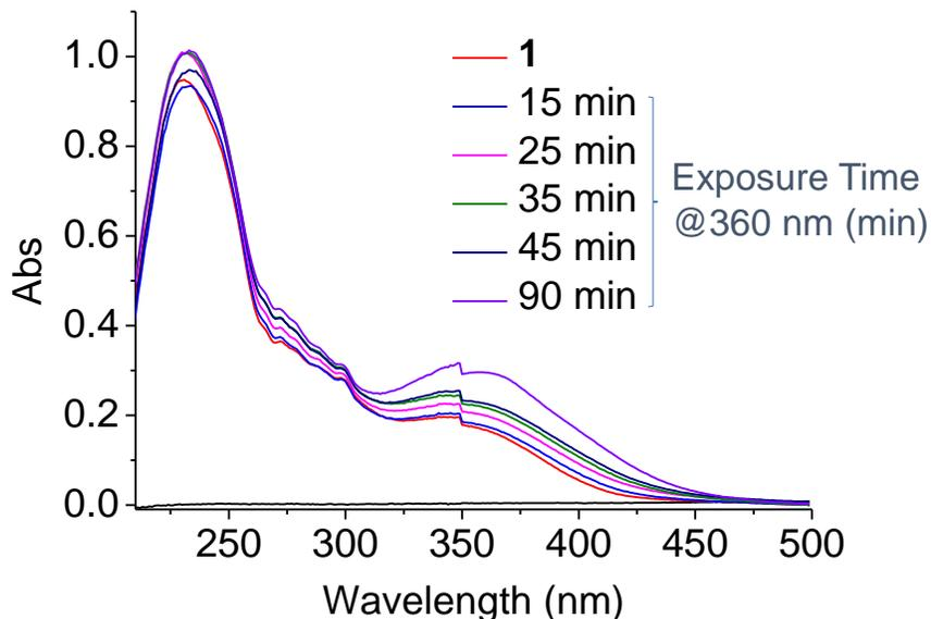
**Figure S1:** UV spectra of **1** after irradiation at 360 nm with increasing times at 360 nm ( $2.7 \text{ mW/cm}^2$ ).
