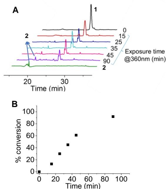
**Figure 1.** **A** HPLC profiles of a 0.5 mM solution of **1** in water at different exposure time at 360 nm ( $2.7 \text{ mW/cm}^2$ ). Elugrams were recorded with 210 nm channel in HPLC. **B** Conversion degree of the photolysis of **1**.
