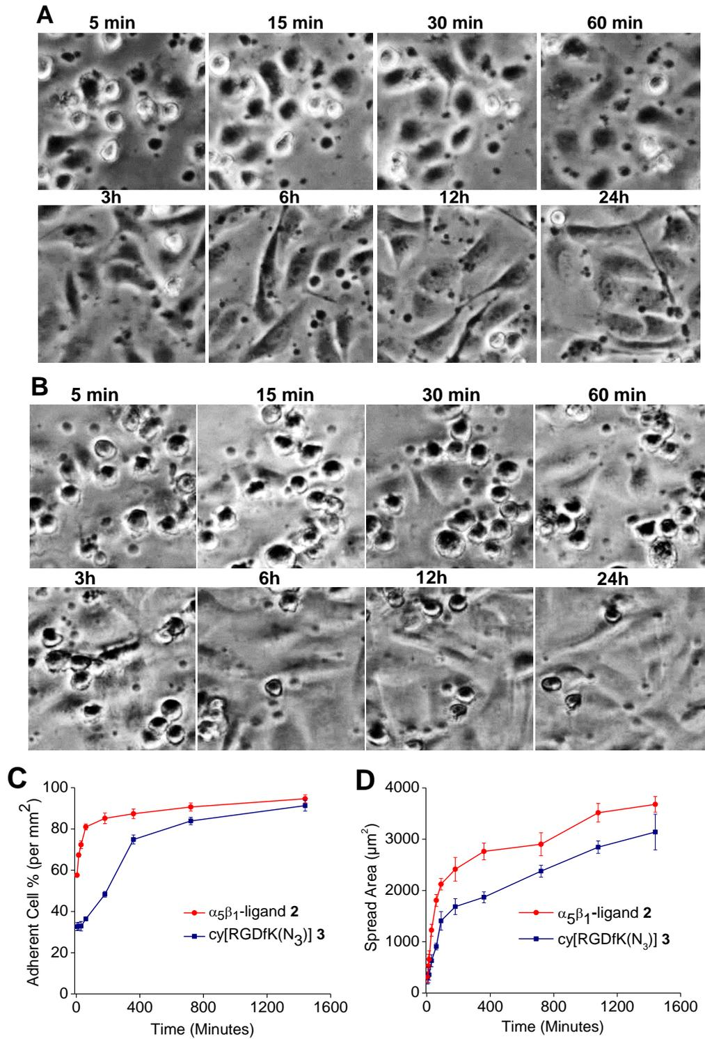
**Figure 3. A, B:** Phase contrast microscopy images of time lapse experiment over 24 hours showing the morphology of HUVECs cultured on Nexterion H slides functionalized with  $\alpha_5\beta_1$ -ligand 2 (A) or cy[RGDfK(N<sub>3</sub>)] 3 (B) ligands (incubation concentration 0.02 mgmL<sup>-1</sup>). **C, D:** Quantification of adherent cells and cell spreading area at different time points..
