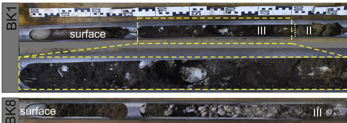
Fig. 13. BK 1 and BK 8 cores from the SQUID magnetic anomaly in the Northern Section. An organic-rich top soil matrix embeds limestone gravels and blocks. The limestones were crushed during vibra-coring (Photos: S. Dietel, 2017).
