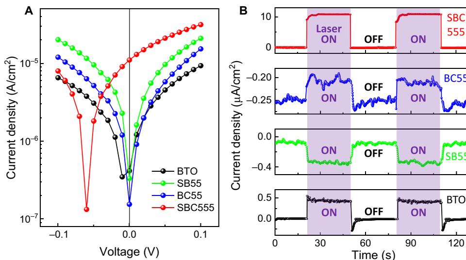
**Fig. 2. Enhancement of photovoltaic effect in tricolor superlattices.** (A) Current-voltage ( $IV$ ) characteristics measured with 3.06 eV at room temperature. (B) Current-time response acquired with the illumination ON and OFF.
