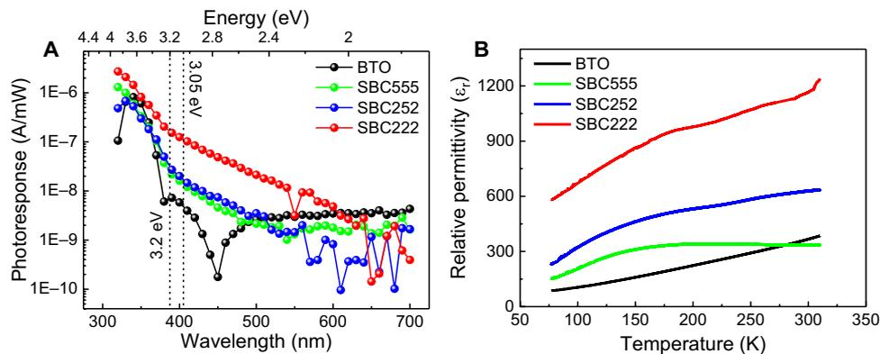
**Fig. 4. Spectral photoresponse and dielectric characterization.** (A) Spectral photoresponse measured at 77 K without any bias voltage. (B) Relative permittivity measured as a function of temperature with an ac signal of amplitude 100 mV and frequency 100 kHz.
