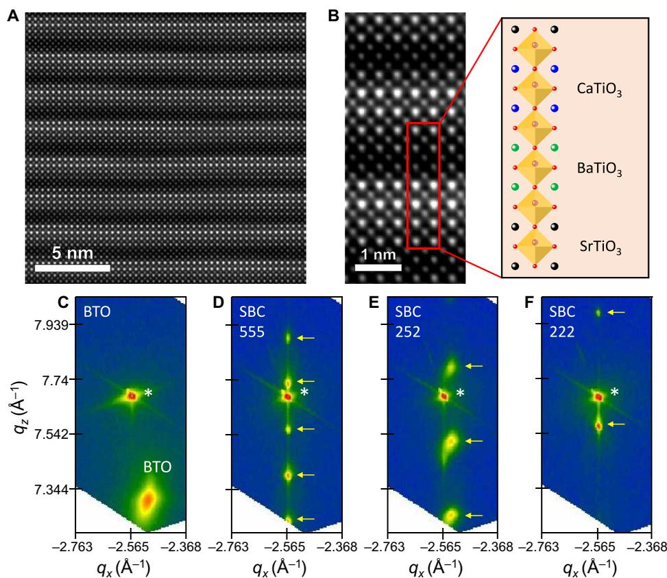
**Fig. 1. Structural characterization of superlattices.** (A) Cross-sectional STEM acquired from sample SBC222. (B) High-resolution STEM from a part of the scanned region. The schematic depicts the arrangement of unit cells. RSM acquired around (103) reflection in (C) BTO, (D) SBC555, (E) SBC252, and (F) SBC222. Star and yellow arrows indicate the STO substrate and satellite peaks from SL, respectively.
