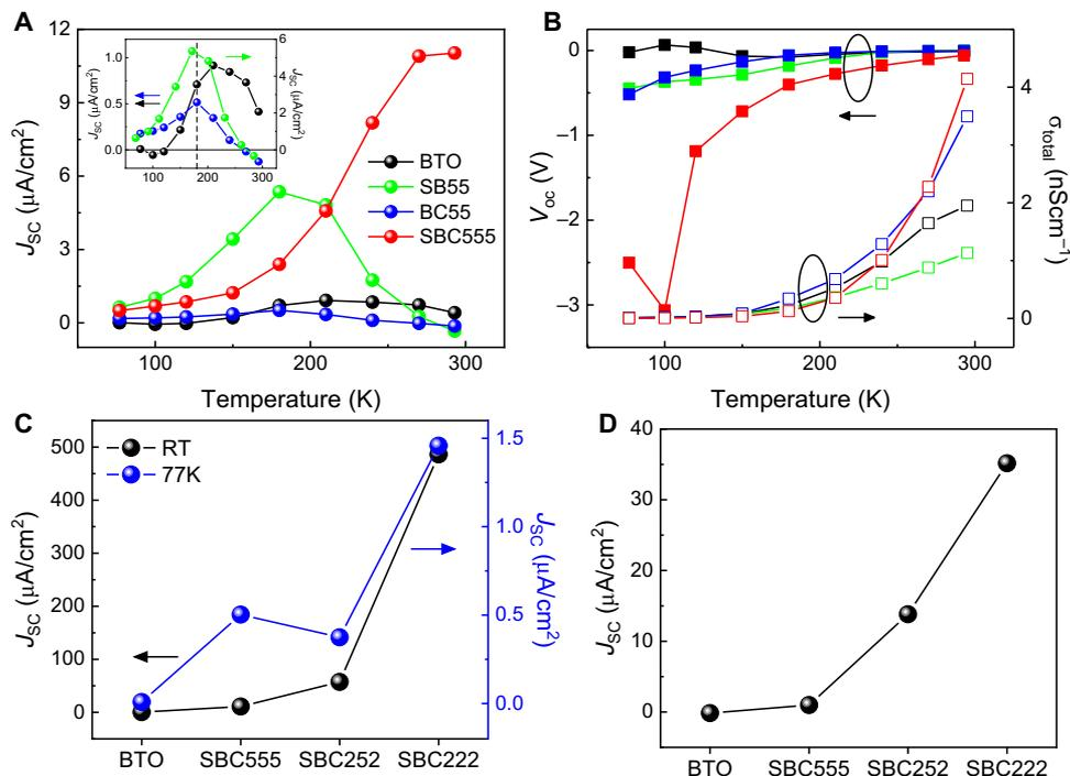
**Fig. 3. Temperature- and periodicity-dependent photovoltaic effect.** (A)  $J_{sc}$  extracted from  $IV$  characteristics acquired at different temperatures. The inset shows vertically magnified curves for BTO, SB55, and BC55. (B) Extracted values of  $V_{oc}$  and  $\sigma_{total}$  as a function of temperature. (C)  $J_{sc}$  measured in different samples at room temperature (RT) and 77 K. (D)  $J_{sc}$  measured under 1.5 AM solar illumination at room temperature.
