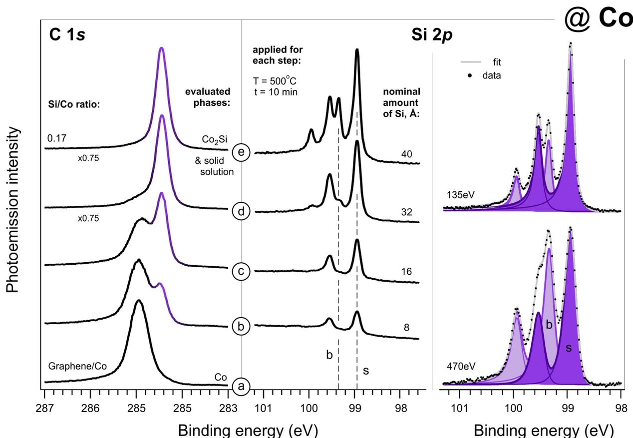
**Figure 6 | Formation of graphene-capped silicides in the Co-based system monitored with XPS.** Evolution of the C 1s and Si 2p spectra with Si intercalation underneath graphene on Co(0001) (left panel). The highlighted part of the C 1s spectra corresponds to decoupled graphene regions. Separation of the silicon atoms embedded in the cobalt layer near the surface and in the bulk obtained via deconvolution of the Si 2p spectrum (right panel).
