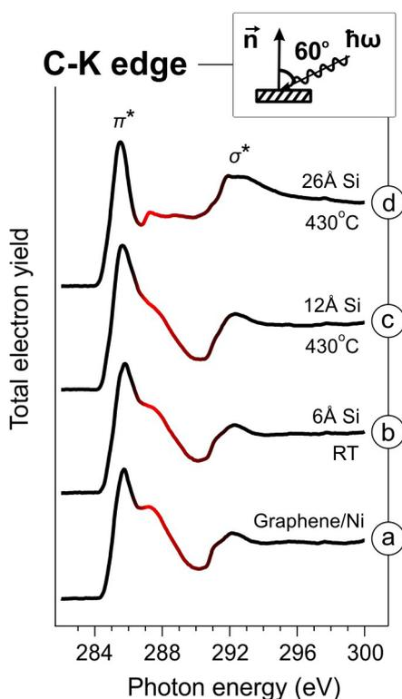
**Figure 4 | Evidence of electronic graphene-substrate decoupling upon silicides formation.** NEXAFS spectra at the carbon K-edge for graphene/Ni(111) (a), and for the systems with intercalated Si (b–d). The part of the spectrum that does not exhibit angular dependence is highlighted in red. The geometry of the experiment is depicted in the inset.
