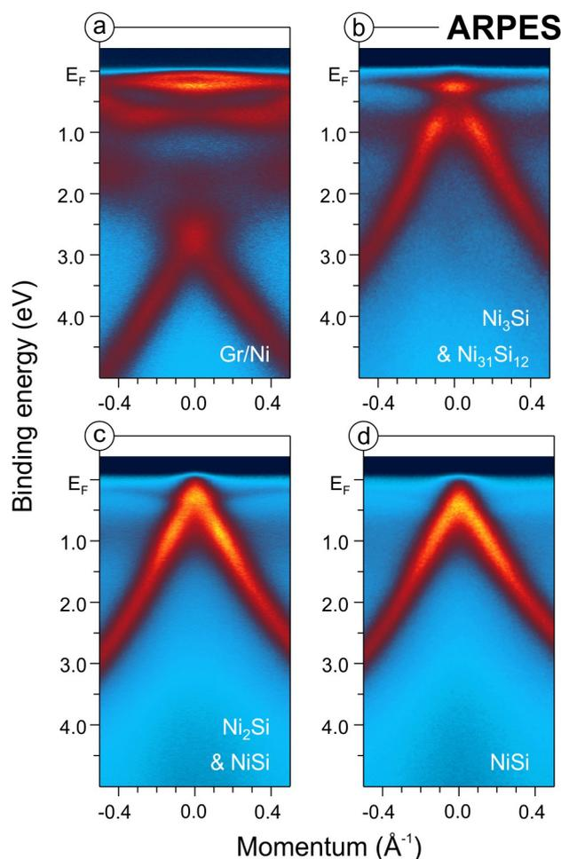
**Figure 5 | Quasi-freestanding character of graphene on silicides.** The sequence of ARPES data for graphene on Ni(111) (a), and at its detachment upon Si intercalation and silicide formation (b–d). The data were obtained near the K-point of graphene Brillouin zone using 40 eV photons.
