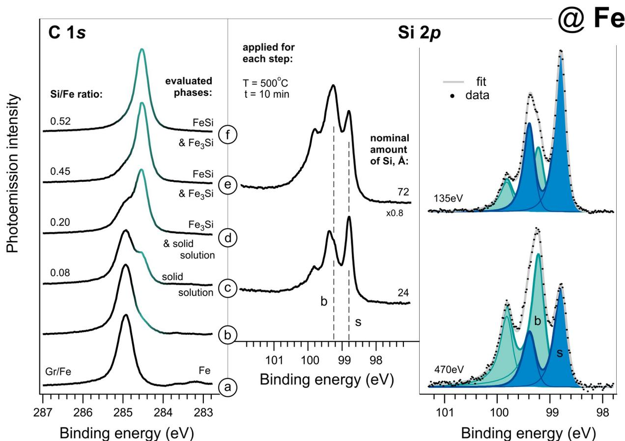
**Figure 7 | Formation of graphene-capped silicides in the Fe-based system monitored with XPS.** Evolution of the C 1s and Si 2p spectra with Si intercalation underneath graphene on a Fe(110) layer (left panel). The highlighted part of the C 1s spectra corresponds to decoupled graphene regions. Separation of the silicon atoms embedded in the iron layer near the surface and in the bulk obtained via deconvolution of the Si 2p spectrum (right panel).
