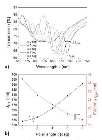
Figure 6. a) Wavelength transmission spectra measured for a tethered structure A as a function of the angle of incidence  $\theta$ . The measurement was done in TE polarization at T = 22 °C (swollen state) for a structure with  $\Lambda = 460$  nm and D = 110 nm. b) Dependence of LSP wavelength position  $\lambda_{\rm LSP}$  and the spectral width (FWHM)  $\Delta\lambda_{\rm LSP}$  on the angle of incidence  $\theta$ .
