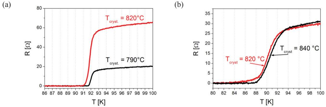
Fig. 2. (a) Measurement of the critical temperature ( $T_c$ ) of (a) YBCO films and (b) GdBCO films, crystallized at different temperatures.
