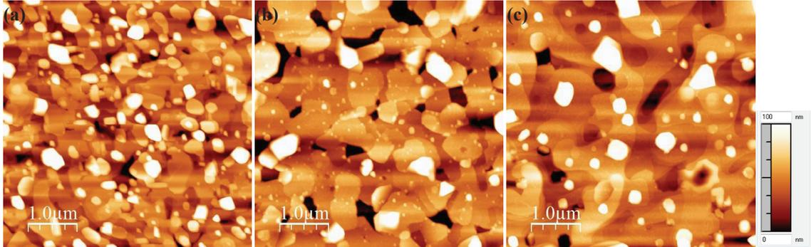
Fig. 3. AFM measurements of (a)  $YBa_2Cu_3O_{7-x}$  (b)  $(Y_{25}Gd_{75})Ba_2Cu_3O_{7-x}$  and (c)  $GdBa_2Cu_3O_{7-x}$  films on a STO substrate crystallized at a temperature of 820 °C.
