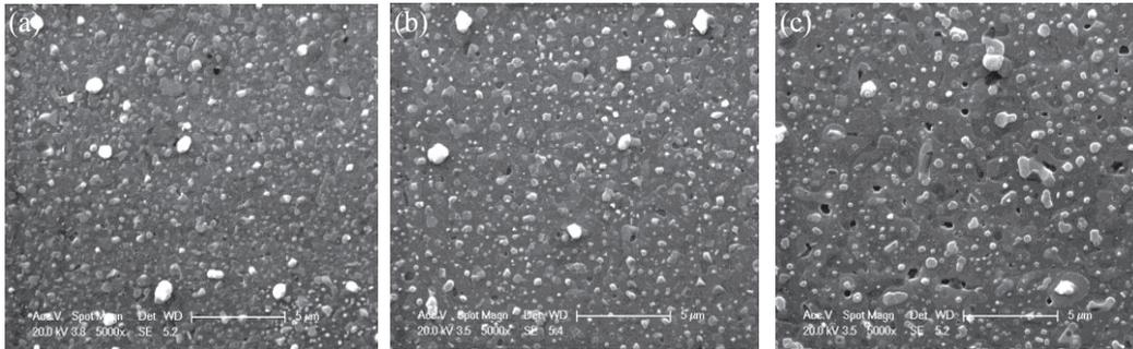
Fig. 4. SEM images of (a)  $\text{YBa}_2\text{Cu}_3\text{O}_{7-x}$  (b)  $(\text{Y}_{25}\text{Gd}_{75})\text{Ba}_2\text{Cu}_3\text{O}_{7-x}$  and (c)  $\text{GdBa}_2\text{Cu}_3\text{O}_{7-x}$  films on a STO substrate crystallized at a temperature of 820 °C.
