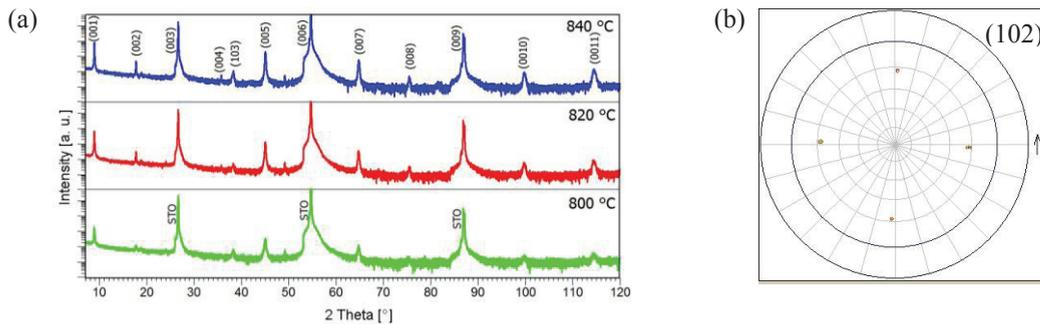
Fig. 1. (a) X-ray diffraction pattern (using Co-K $\alpha$  radiation) of GdBCO films deposited on SrTiO<sub>3</sub> prepared from water-based precursor solution annealed at different crystallization temperatures; (b) YBCO (102) pole figure of a film annealed at a crystallization temperature of 800 °C.
