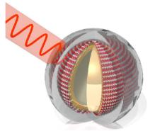
Figure 19. Sketch of an SERS nanotag comprising a hollow Au/Ag nanoshell coated with an SAM of an aromatic thiol as the Raman reporter molecule. The particle is protected by a silica shell. Rerproduced with permission from ref 327. Copyright 2009 Wiley-VCH.
