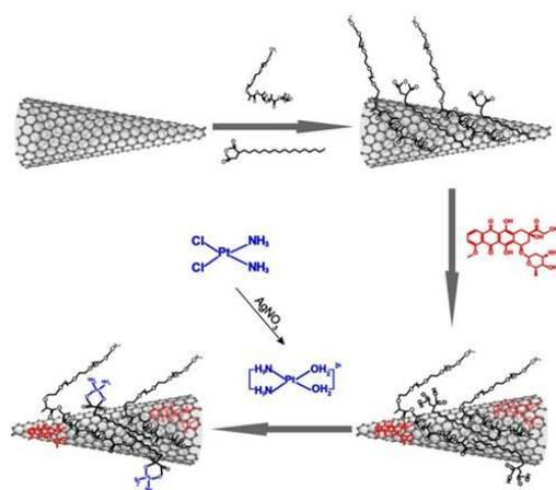
**Figure 4.** Schematic representation of the preparation of Cisplatin and Doxorubicin dual loaded Single-Walled Carbon Nanohorns. Reproduced from [100]. Ivyspring (2018).
