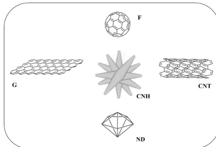
**Figure 1.** Representation of the main carbon nanostructures.
