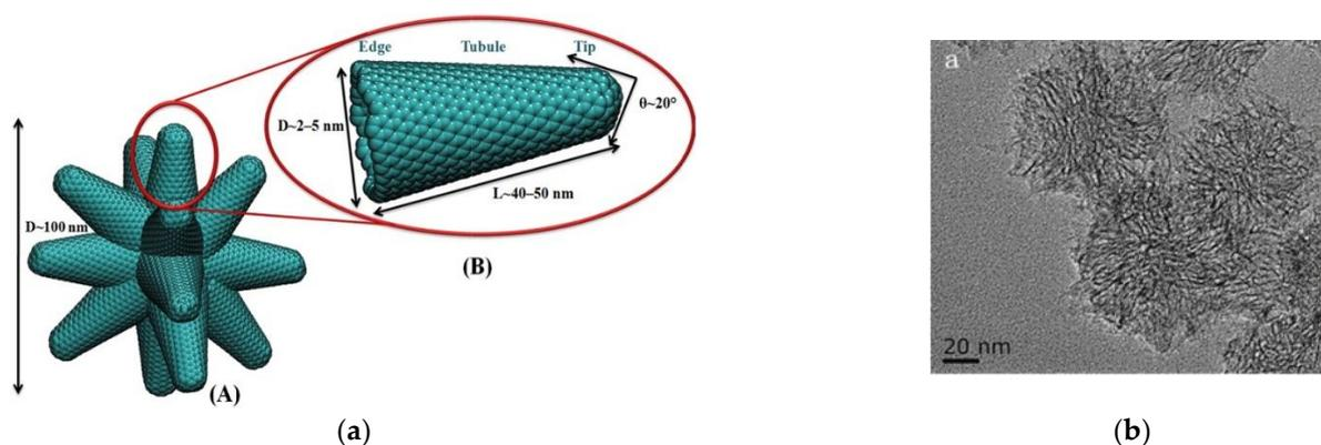
**Figure 2.** (a) Schematic representation of the morphological features of (A) dahlia like Carbon Nanohorns (CNH) and (B) single CNH, reproduced with permission from [63], Elsevier (2019). (b) Representative TEM image of dahlia like CNH. Reproduced with permission from [64], Elsevier (2015).
