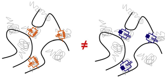
Fig. 25. Schematic representation of the differences between the conductivity ('electrical network') and rheological properties (mechanical active filler network): The shaped nanotubes are represented by black lines and the polymer chains by gray lines. To symbolize the contact resistance an 'electrical equivalent circuit' was taken, whereas the viscoelastic coupling between CNTs via polymer chains is represented by a 'dash pot' for local friction and an 'entropic spring'.
