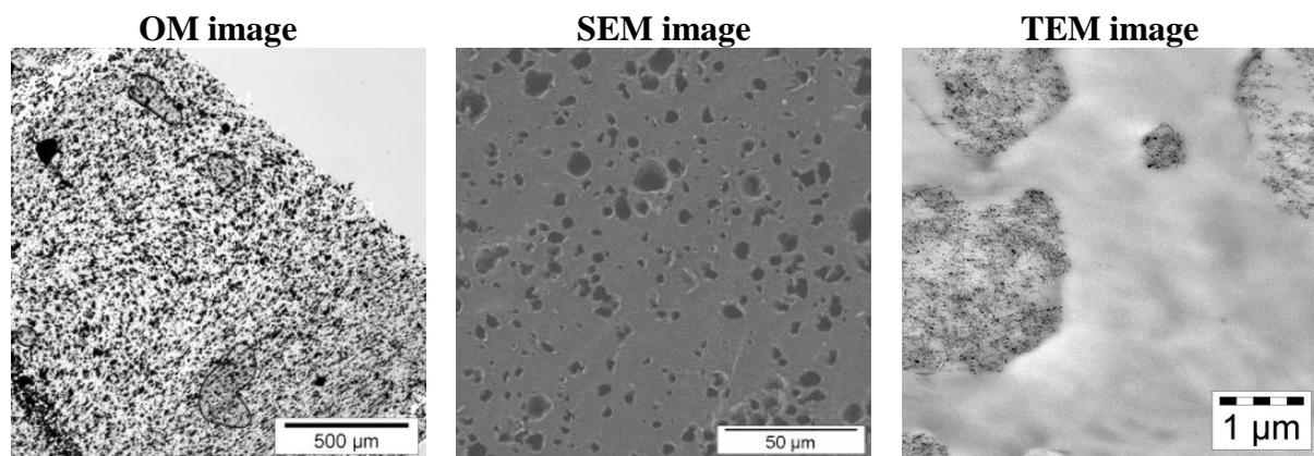
35 *Figure 3.* Microscopy images of PC22: transmission optical micrograph of a thin section
