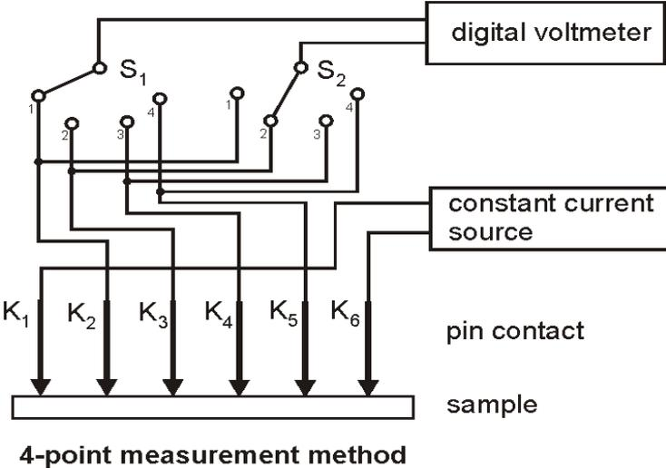
Figure 2: Resistance measurement setup.
