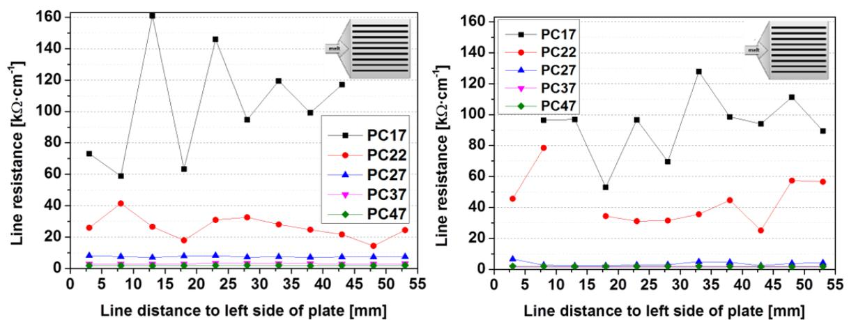
49 *Figure 5.* Resistance of lines as function of line position in flow direction and blend
