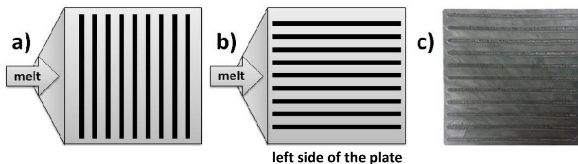
*Figure 1.* a) Schema for the arrangement of the laser lines when irradiated (a) perpendicular to melt flow direction, b) in melt flow direction with the injection gate on then left hand side and c) photograph of a real sample ( $60\times 60\text{mm}^2$ , thickness 2.5 mm).
