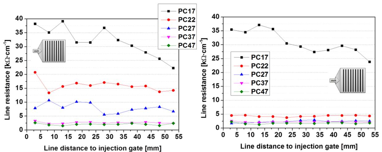
54 *Figure 4.* Resistance of lines as function of line position perpendicular to flow direction at
