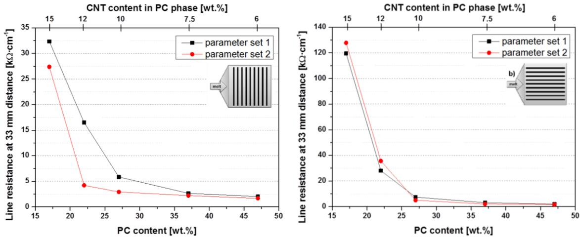
25 *Figure 6.* Line resistances at position 33 mm as function of PC content: perpendicular to melt
