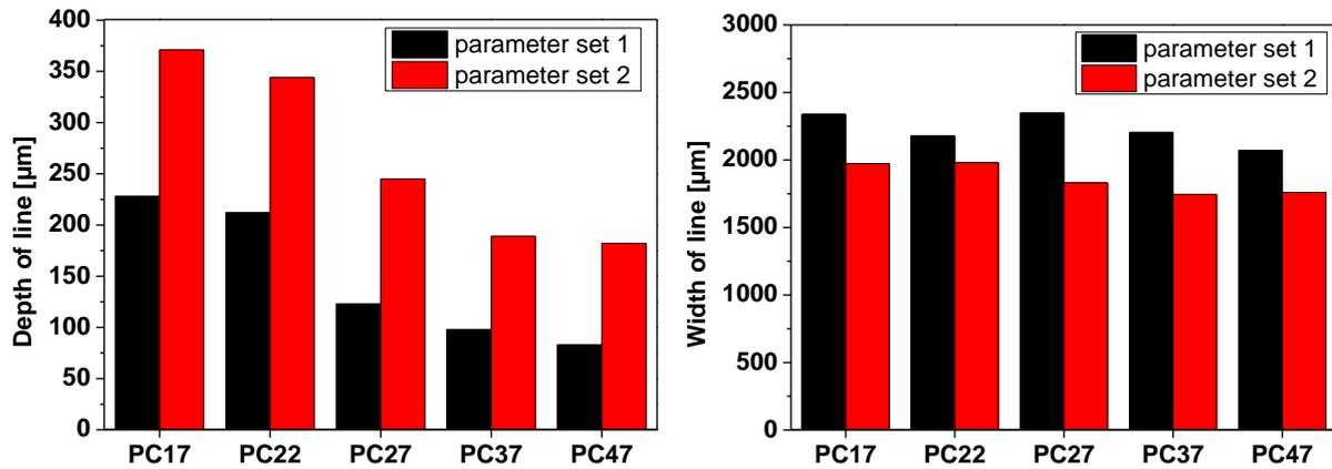
Figure 9. Geometric dimensions depth and width of the created conductive tracks at different blend compositions.
