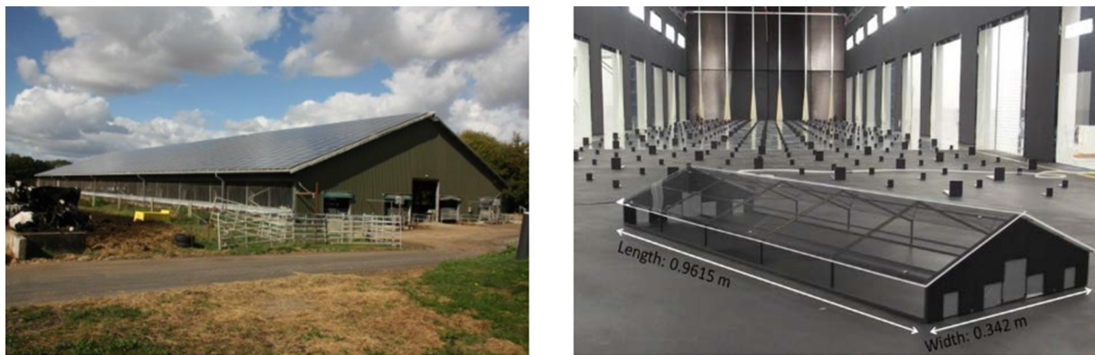
Fig. 1. Left: Real scale barn. Right: 1:100 scale model in the wind tunnel.
