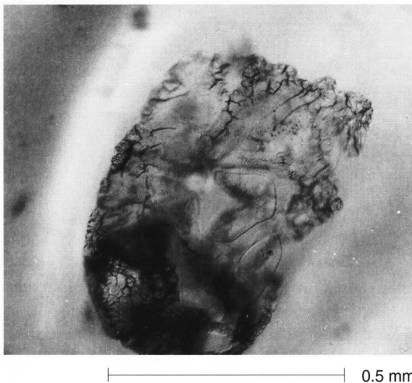
Figure 7. Nepheline remnant close to the surface of a crystal glass surface investigated under transmitted polarized light.
