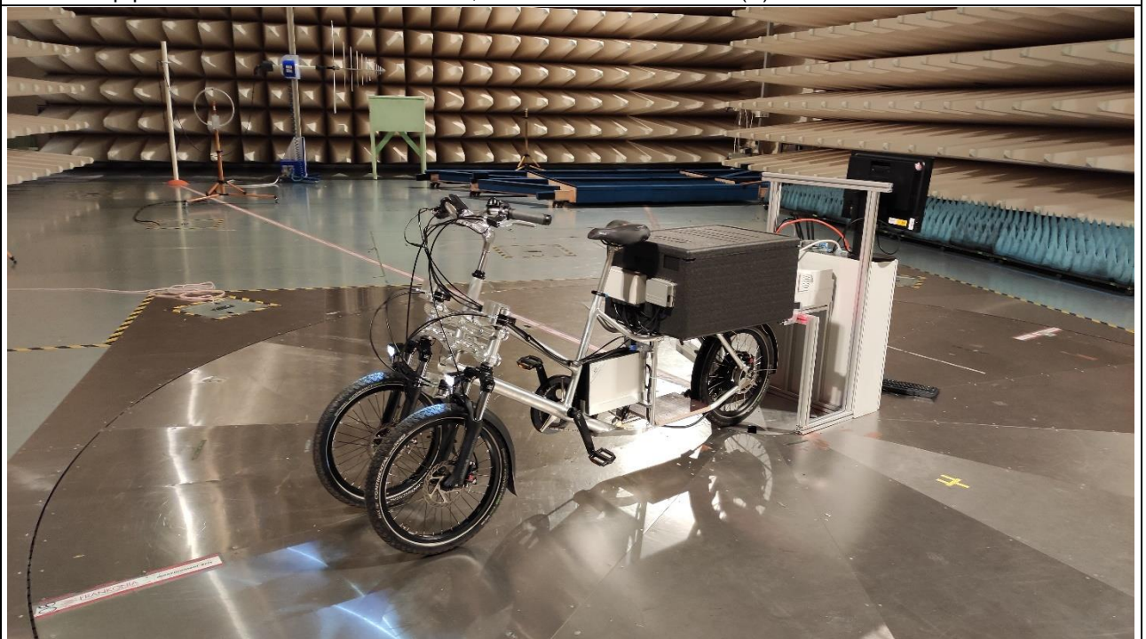
Test set-up photo: Orientation 0° of the DUT, Antenna orientation 90° (Y)
