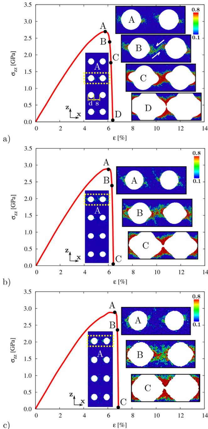
**Fig. 1.** MD simulations: Tensile stress–strain curves together with snapshots of the local atomic shear strain along the deformation of three nanoporous BMGs with pore sizes of 18 (a), 9 (b) and 4.5 nm (c), respectively. For a better visualization of the deformation mechanism only the line of pores along which the structures deform is shown (regions with yellow boundaries).
