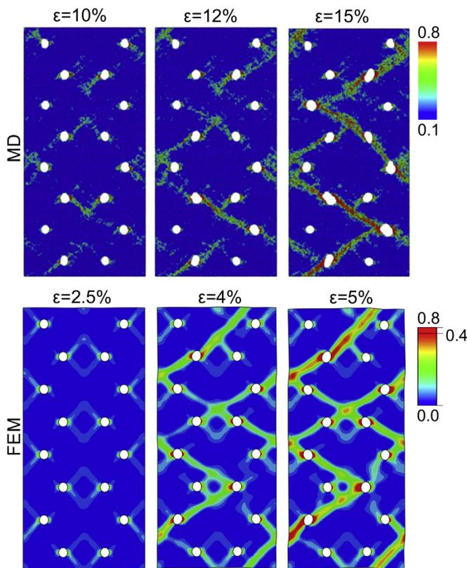
**Fig. 5.** Local atomic shear strain and the equivalent plastic strain distributions at different strain levels under tensile deformation of the nanoporous BMG with pores of 2.6 nm and a honeycomb-like pore distribution.
