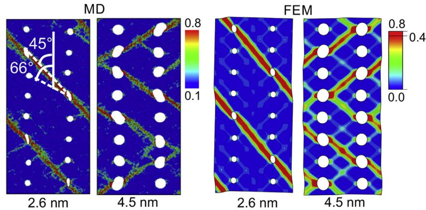
**Fig. 4.** Local atomic shear strain from MD simulations and equivalent plastic strain distributions from FE simulations of the heterostructure with pores of 2.6 nm and 4.5 nm. Both methods reveal similar plastic behavior under tensile deformation.
