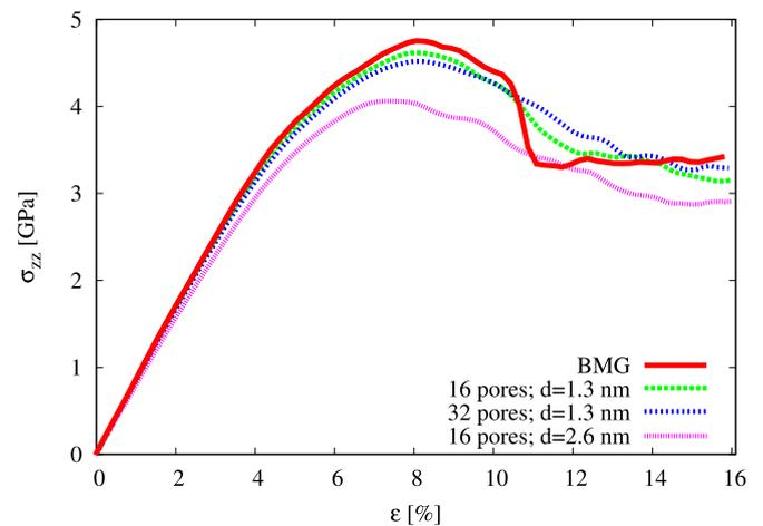
**Fig. 6.** Tensile stress–strain curves of two nanoporous BMGs with 16 pores of 2.6 nm and 1.3 nm and one with 32 pores of 1.3 nm in comparison with a monolithic BMG at a strain rate of  $4 \cdot 10^7 \text{ s}^{-1}$ .
