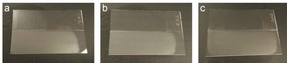
Figure 5. Visual demonstration of the anti-fog effect of a) MPC 4% @SiO 2 (glass), b) MPC 2% @SiO 2 (glass), and c) MPC 1% @SiO 2 (glass). The images present in each case the comparison of a coated glass sample (upper slide) with a nonfunctionalized one (lower slide).
