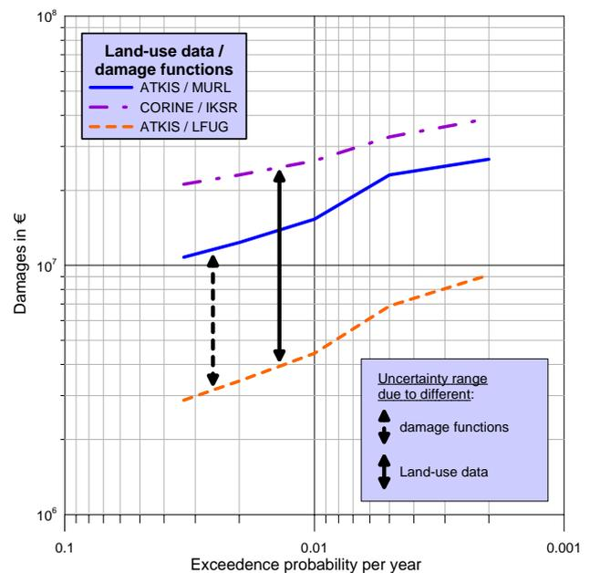
**Fig. 3.** Total flood damages for return periods up to 500 years for the community of Meissen on the Elbe River in Germany. Calculations are based on different damage functions and land-use data. (source: Herrmann et al., 2007<sup>1</sup>).
