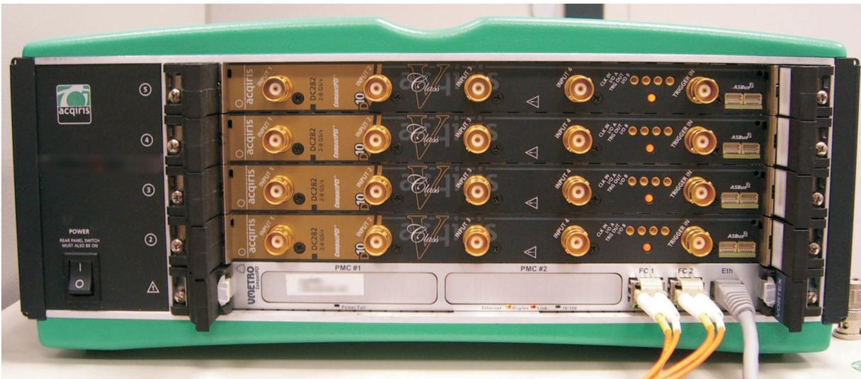
**Figure 2.3:** Crate with four digitizer cards (upper slots) and one recording card (VMETRO, lower slot). The nELBE FDDAS consists of two of these crates and two JBODs (see text for details).
