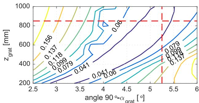
**FIG. 2.** The average spectral resolution (in eV) within 12–41 nm is plotted for different source-to-grating distances  $z_{\text{grat}}$  and grating incidence angles  $\alpha_{\text{grat}}$ . The optimum working point for our XCT setup is indicated with the red dashed cross. The spectral resolution for this geometry is below  $\Delta E < 0.04$  eV.
