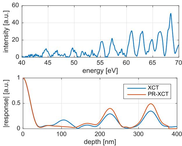
**FIG. 6.** Upper graph: The plot shows the spectral modulation of the sample measured by the T-REXS. Lower graph: The retrieved depth signal of two gold layers buried under silicon including the autocorrelation artifacts (blue) is shown. The use of the phase retrieval algorithm of XCT removes the autocorrelation artifacts near 100 nm (red). The gold layers are located at 230 nm and 330 nm. An oxide layer is found at 160 nm.
