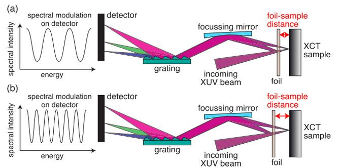
**FIG. 7.** Principle of the broad bandwidth resolution test: (a) A thin foil is placed in front of a silicon wafer. A small foil-to-surface distance introduces slow spectral oscillations in the spectrometer. (b) Larger foil-to-surface distances lead to faster spectral oscillations. For increasing distances, the resolution  $\mathcal{R}(k)$  reduces the ability to resolve the fast oscillations. A scan of the foil-to-surface distance allows a measurement of the FTR.
