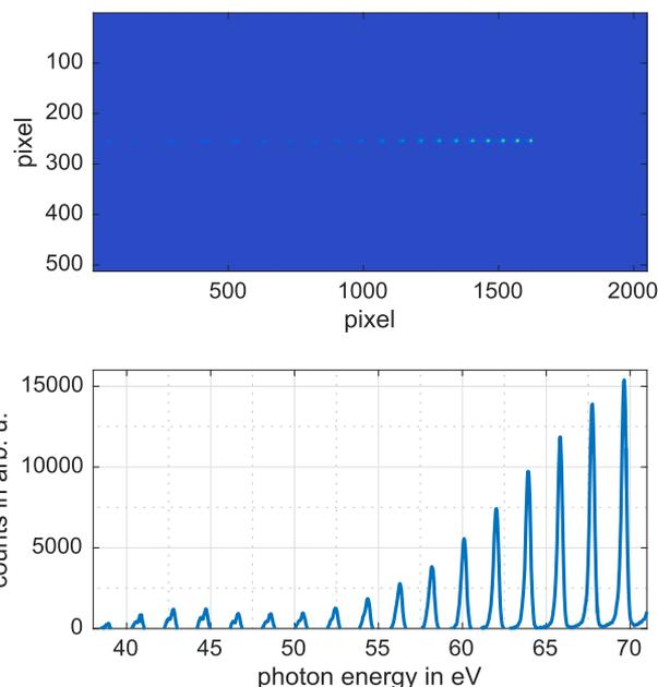
**FIG. 5.** A HHG spectrum is recorded using the focusing mirror and the 1300 nm driving laser. The XUV beam is focused down to a few pixels on the CCD camera. This leads to a short exposure time of 0.6 s. This operation mode has the highest sensitivity and is typically used for XCT measurements.
