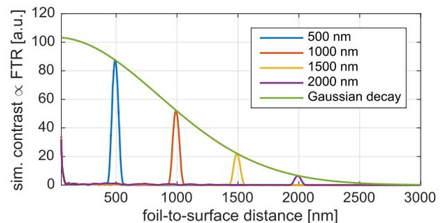
**FIG. 8.** A simulated FTR and the decay of the simulated contrast for different foil-to-surface distances are shown (500, 1000, 1500, and 2000 nm). Due to the finite resolution of a spectrometer, the signal decreases with increasing distance. The FWHM width  $\Delta x = 2 \mu\text{m}$  of the FTR corresponds to a resolution of  $\overline{\Delta E} = 0.087 \text{ eV}$ .
