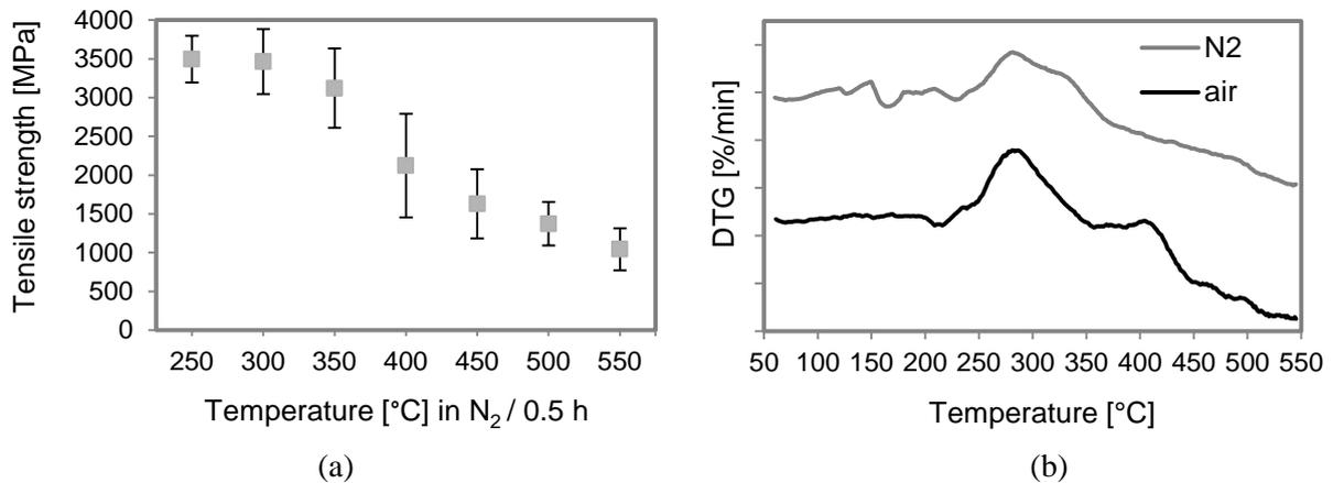
**Figure 3.** (a) Single fibre tensile strength of sized basalt fibres after 0.5 heat treatment in nitrogen atmosphere (b) TGA/DTG curves of sized basalt fibres.
