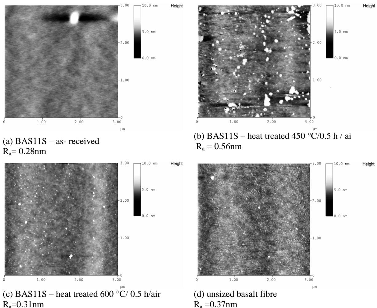
**Figure 5.** Fibre surface and arithmetic surface roughness  $R_a$  of as-received (a), heat treated (b), (c) and unsized basalt fibres (d).
