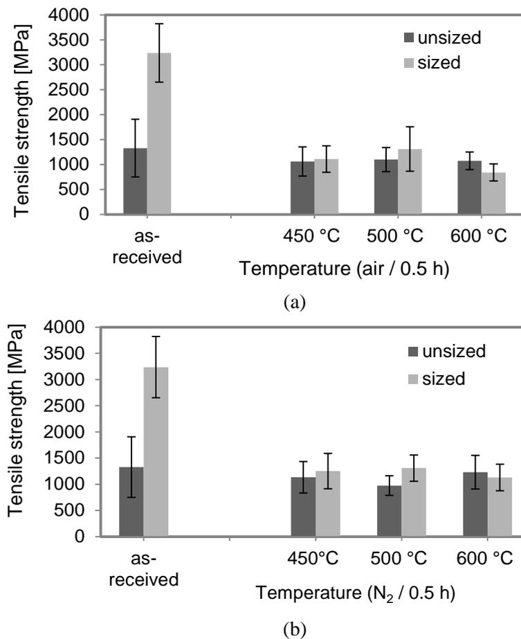
**Figure 4.** Single fibre tensile strength of unsized and sized basalt fibres after heat treatment in air (a) and in nitrogen atmosphere (b).
