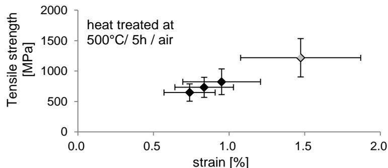
**Figure 2.** Tensile strength-strain behaviour of heat treated basalt fibre samples; (gray diamond indicates unsized BAS11 sample).
