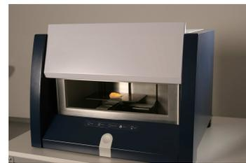
M4 Tornado High performance micro XRF spectrometer
