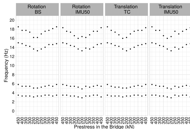
Figure 50: Variation of first four eigenfrequencies of the BLEIB structure under different prestress conditions obtained from conventional TC and BS sensor and 6C IMU50 sensors placed at location 3.
