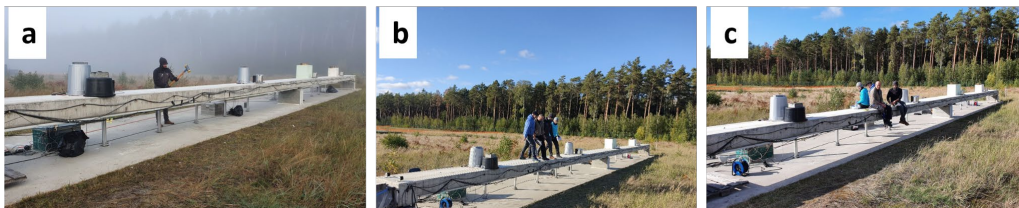
Figure 18: During the active tests: the impulsive excitation by hammer hitting (a), the vertical harmonic excitation generated by approx. 1 Hz squats (b) and the static load approx. 280 kg at SP2 (c).
