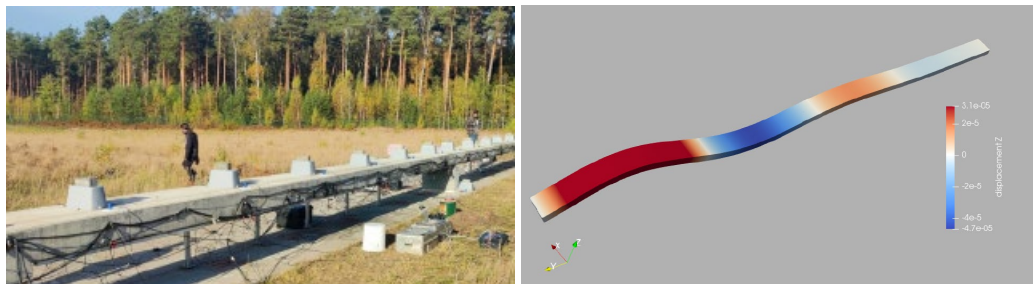
Figure 2: The newly developed GIOTTO IMU50 sensor network installed at the BLEIB test structure (left panel) and the simulation of the 6C wavefield in a digital twin implemented in Salvus (Mondaic, Switzerland).
