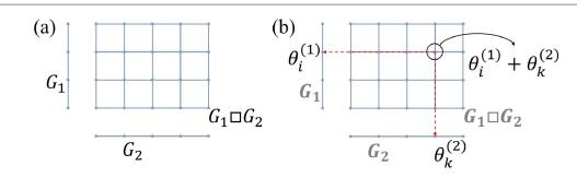
**Figure 1.** Panel (a): Cartesian product of two factors (chains)  $G_1$  and  $G_2$ . Panel (b) product of two phase oscillators using the Kronecker sum.
