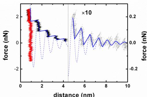
**Figure 3** Comparison of data from figure 1 with a model in which the potential is calculated as integral over the tip-sample gap area of exponentially decaying oscillatory contributions (see text for details). The dashed blue line shows the model force curve, the solid blue line the expected force-distance approach curve for the cantilever stiffness of  $k = 0.15$  N/m, and the dots are experimental data points, black dots for approach and red dots for retraction.
