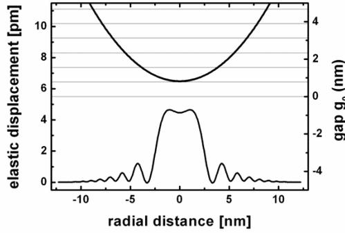
**Figure 4:** Combined elastic displacement  $g(r) - g_0 - r^2/(2R_c)$  of tip and surface for one double layer of ionic liquid confined between tip and surface and a normal force of 2 nN. The upper part of the graph shows the gap  $g(r)$  for comparison. The lines indicate the distance between double layers of ionic liquid.
