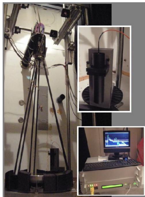
Fig.2: Installation of the NARLa receiver/detection unit next to the KARL lidar receiver at Ny-Alesund.
