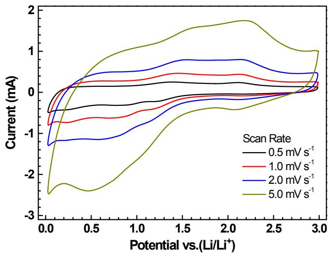
**Figure S5.** Cyclic voltammetry results for the PCC-CoO<sub>x</sub> electrode at various sweep rates in the potential window of 0.01-3.0 V.
