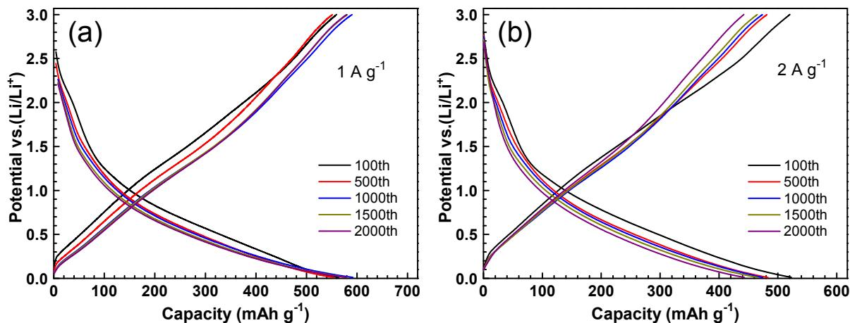
**Figure S6.** Discharge/charge voltage-capacity profiles of the PCC-CoO<sub>x</sub> electrodes at (a) 1 A g<sup>-1</sup> and (b) 2 A g<sup>-1</sup>.
