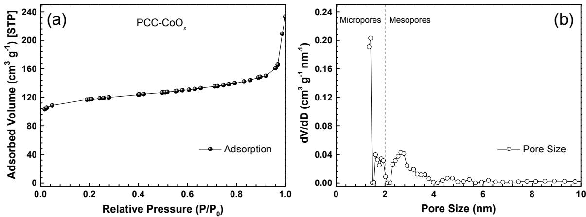
**Figure S3.** (a) Nitrogen physisorption isotherm, and (b) the corresponding pore size distribution curve obtained from the adsorption branch by applying non-local density functional theory (NLDFT) for the PCC-CoO<sub>x</sub> sample.
