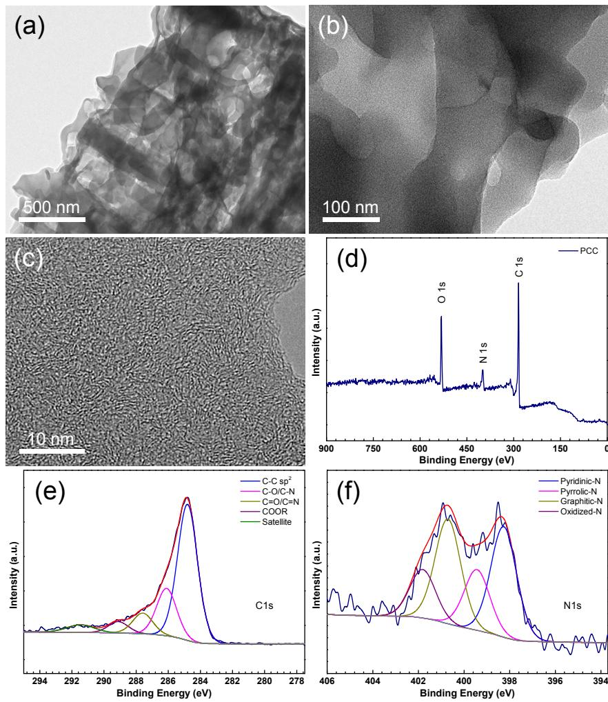
**Figure S1.** Morphology images and XPS spectra of the PCC sample. (a) and (b) TEM images; (c) high-resolution TEM image. (d) Full XPS spectrum containing C, O, and N; (e) high-resolution of C 1s spectrum, and (f) high-resolution of N 1s spectrum.
