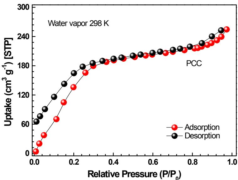
**Figure S2.** Water physisorption isotherms at 25 °C of the PCC sample.
