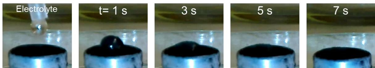
**Figure S7.** Time-lapse photographs of the electrolyte droplet (1.0 M LiPF<sub>6</sub> + EC/DEC/DMC) on the PCC-CoO<sub>x</sub> sample.
