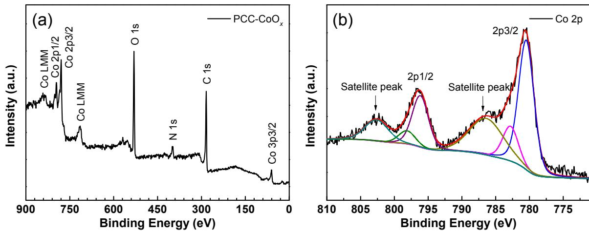
**Figure S4.** (a) Full XPS survey of the PCC-CoO<sub>x</sub> sample containing C, Co, O, and N. (b) High-resolution of Co 2p spectrum (Co<sup>0</sup> and Co<sup>2+</sup>).
