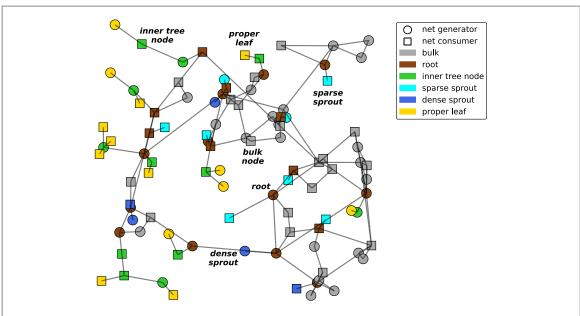
**Figure 1.** Spatially embedded representation of one random synthetic power grid with N = 100 nodes of which half are net generators and half net consumers. Nodes are coloured according to their topological class, see section 2.3 for definitions.
