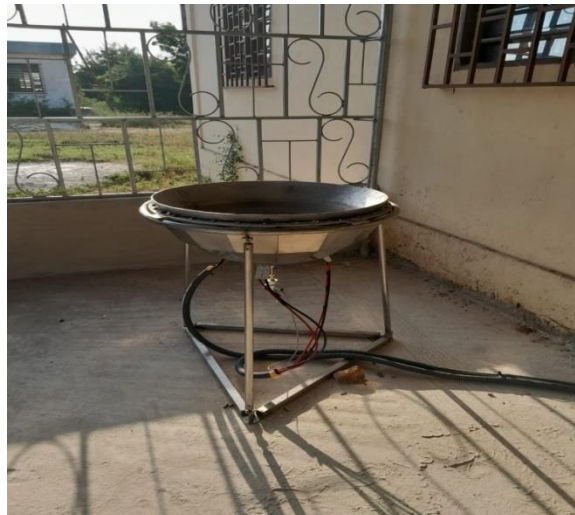
Figure 4: Direct Solar PV powered gari roasting pan
