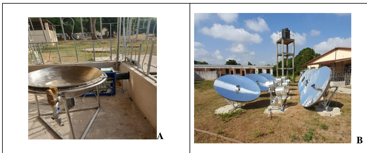
Figure 5 (A) SCSP reflector steam powered roasting pan and (B) Scheffler Concentrated Solar Power Reflectors (SCSP) for the steam powered roasting pan
