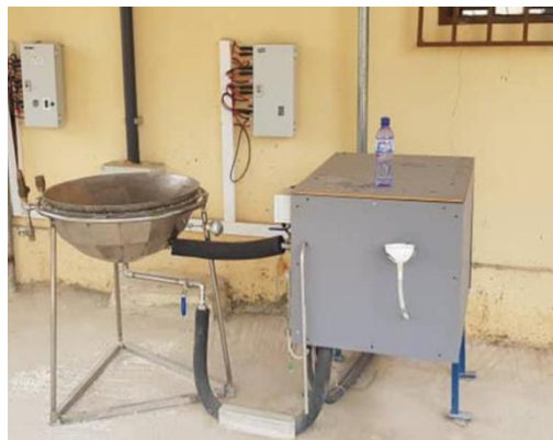
Figure 6: Solar PV-steam powered gari roasting panel
